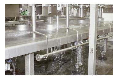
FIGURE 26.2 All surfaces in the product zone are designed to be self-draining for liquid food, cleaning and disinfection solutions, and rinsing water. *Courtesy of Krones AG*.
