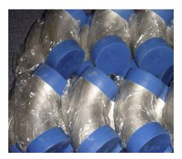
FIGURE 26.58 Stainless steel equipment components should be (shrink) wrapped with plastic film to protect them against corrosion in contact with black steel (particles), and their inlet and outlet connections should be fitted with protective caps to prevent ingress of impurities, insects and small animals. *Courtesy of Zhejiang Jugang Pipe Co., Ltd.*
