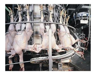
FIGURE 7.2 Automatic equipment used for poultry evisceration. A high-speed broiler line processes a few thousand birds per hour. *Courtesy of Marel – Stork Poultry Processing*.
