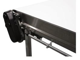
FIGURE 26.33 Motors should rather be located below the line of the product flow. Gears, chains and motors of belt drives must be covered to avoid any contamination of product. However, a chain guard (essential from an occupational safety point of view), when open, may provide a place where product may accumulate, allowing microbes to multiply to large numbers and so posing a contamination risk for the food product on the belt. *Courtesy of Dorner Conveyors*.
