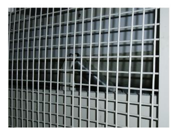
FIGURE 26.37 Example of a hygienically designed guard. Courtesy of P.T. Group.
