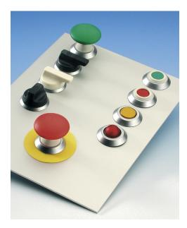
**FIGURE 26.39** Control panel with hygienic control and indicator devices. Seals should fill the gaps between the fixed and moving device parts, to avoid the ingress of product residues, lubricants and organic materials. A perfect, hermetic seal is also required to prevent the ingress of moisture, dust and dirt within the control panel. Adequate space should be provided between control and indicator devices for easy cleaning. *Courtesy of Elan-Schmersal.*
