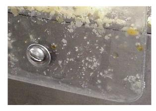
FIGURE 26.3 Product contact surfaces of this equipment are not readily accessible for manual cleaning and disinfection. Moreover, the dome screw with drive slot and washer creates gaps and crevices where debris collects. *Courtesy of Joe Stout, American Meat Institute.*
