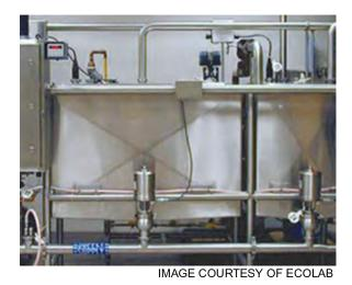
FIGURE 27.1 CIP cleaning solution and sanitizing solution tanks: this single-use CIP system includes two medium-sized tanks for detergent and rinse/sanitizer, a steam heat exchanger, and programmable logic controllers to automate the cleaning process.
