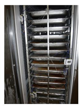
FIGURE 20.2 Simple batch air-cooling system for cooling trays of product.
