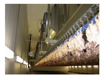
FIGURE 20.3 Continuous air-chilling system for whole poultry.
