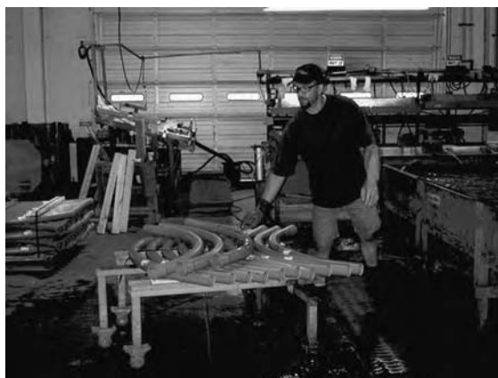
FIGURE 3.21 The ergonomics committee designed this knee-height cart to reduce bending of the back.
