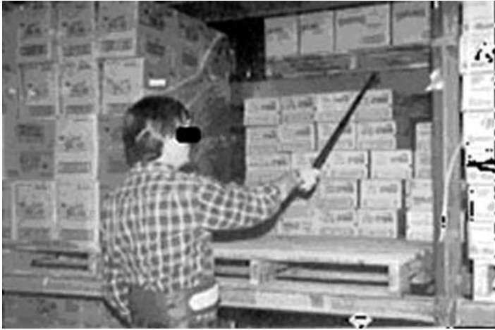
FIGURE 45.23 A pick stick used by a selector to grab a hard-to-reach case.
