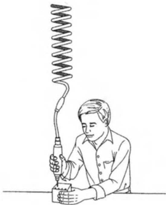
FIGURE 11.5 Balancers permit operators to move loads (typically handtools) around a workstation as if the load had only a small weight. (From Hanna, S. and Konz, S. 2004. Facility Design and Engineering , 3rd ed., Holcomb Hathaway, Scottsdale, AZ. With permission.)
