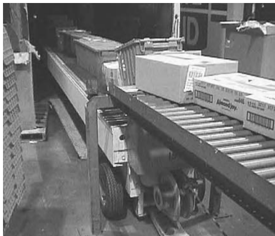
FIGURE 16.23 A boom conveyor is projecting into a truck. As the truck fills, the boom is moved back under the fixed roller conveyor.
