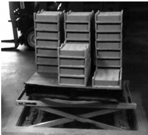
FIGURE 16.16 A recessed lift table has a turntable so that the heavy units can be placed on the side close to the work area. Skirts are available, and should be present, to enclose the open area and reduce the risk of toes being caught under the lift.
