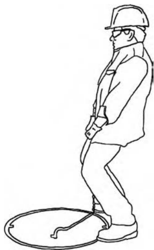
FIGURE 14.A1 A worker removing a manhole cover using a hook and chain.
