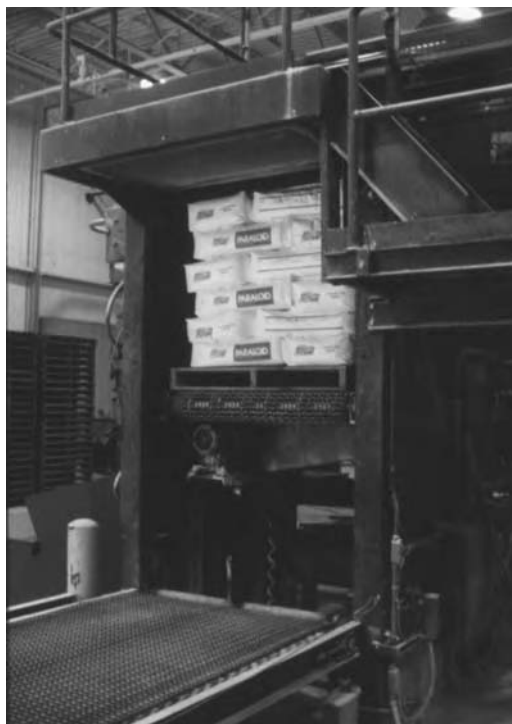
FIGURE 16.1 An autopalletizer for sacks eliminates manual lifting.
