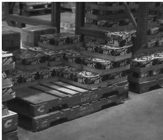
FIGURE 45.6 Raising a pallet in a full slot, by stacking empty pallets under the cases.
