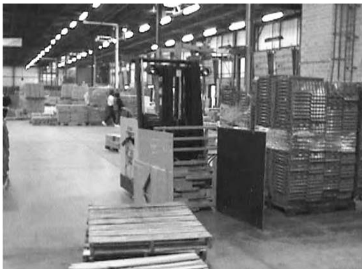
FIGURE 45.13 Mechanical load splitter with a clamping device, used to break down pallets.
