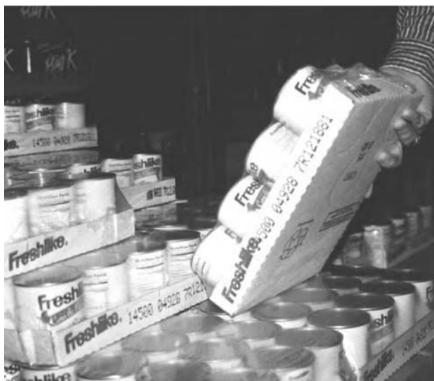
FIGURE 45.10 Tray packs without plastic wrapped on the bottoms of the cardboard trays.
