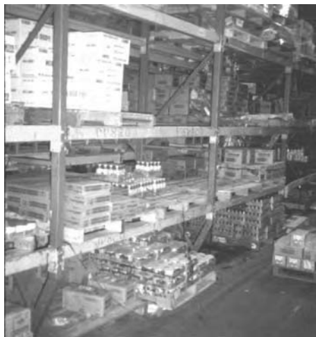
FIGURE 45.12 Example of a triple slot, which requires more extreme body positions of selectors to reach cases.
