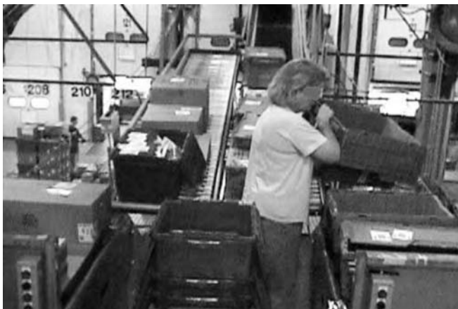
FIGURE 16.11 One employee operates a stacking station with two feed conveyors, each going to a pallet on a high scissor lift. The stacking of the totes is at waist height. The pallet can be filled to the height of a truck without a change in stacking height for the employee. Note the person that is standing down at the ground level, illustrating how high these lifts are from the floor.
