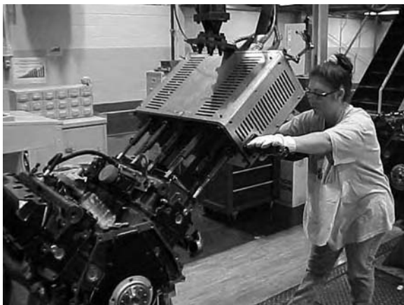
FIGURE 28.2 A multiple spindle bolt runner replaces hand tools used for tightening and torquing bolts.
