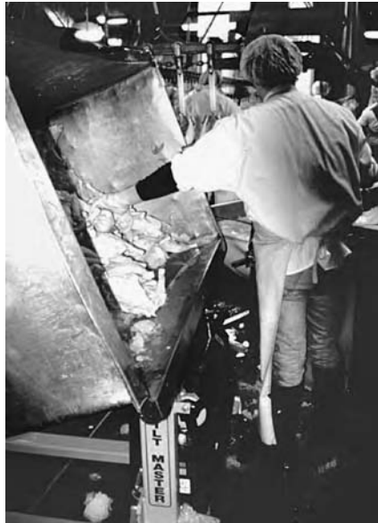
FIGURE 16.14 The product is tilted so that it is closer to pick up. A tank tilter such as this also raises the product to waist height. The reduction in fatigue on the worker improves the performance of unloading the tank.
