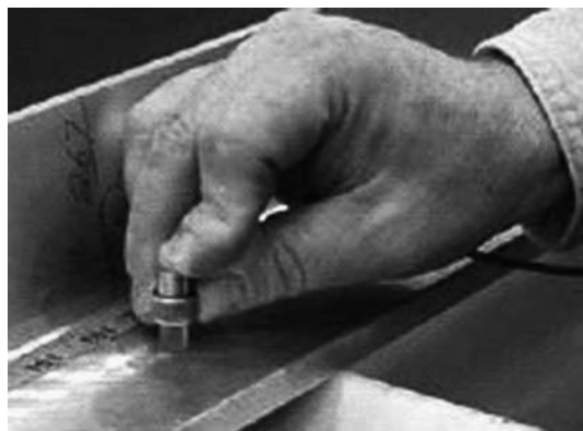
FIGURE 3.16 Before: Quality inspectors frequently used small-diameter gauges requiring forceful pinch grips. (From Boeing Commercial Airplane Group Seattle, WA 2003 and Zawitz Ben, Ergonomics at Boeing . Ergosolutions magazine July/August 2003. With permission.)
