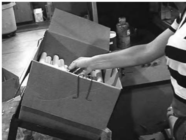
FIGURE 13.6 Tilted box with clips to reduce wrist bending.
