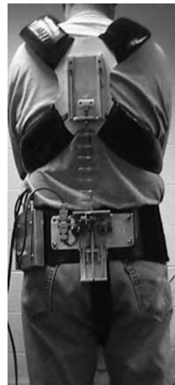
FIGURE 37.1 Lumbar motion monitor.
