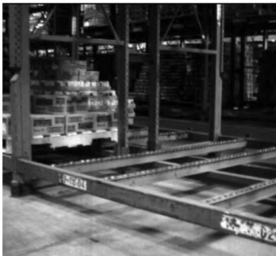
FIGURE 45.7 Using full-pallet flow racks (on rollers) to raise pallets off the floor.
