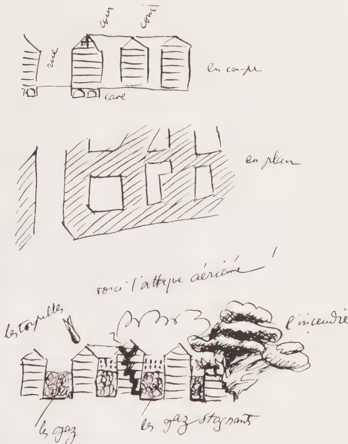
Plate 1.2 Le Corbusier's 1933 Ville Radiuse designs for apartment blocks and cities, which minimized the risks of aerial bombing and gas attack. These are contrasted with the supposed vulnerabilities of traditional, dense, urban streetscapes (see plate 5.1). Source: Le Corbusier (1933: 60–1).
