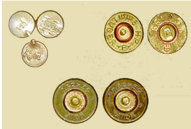
Figure 14.3 Examples of cartridge headstamps.
