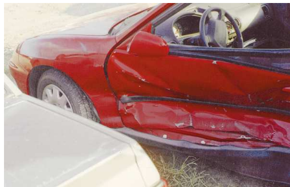
Figure 18.7 Paint transfer marks in contact are “tag” marks and can be chemically compared to the other vehicle to confirm who hit whom.
