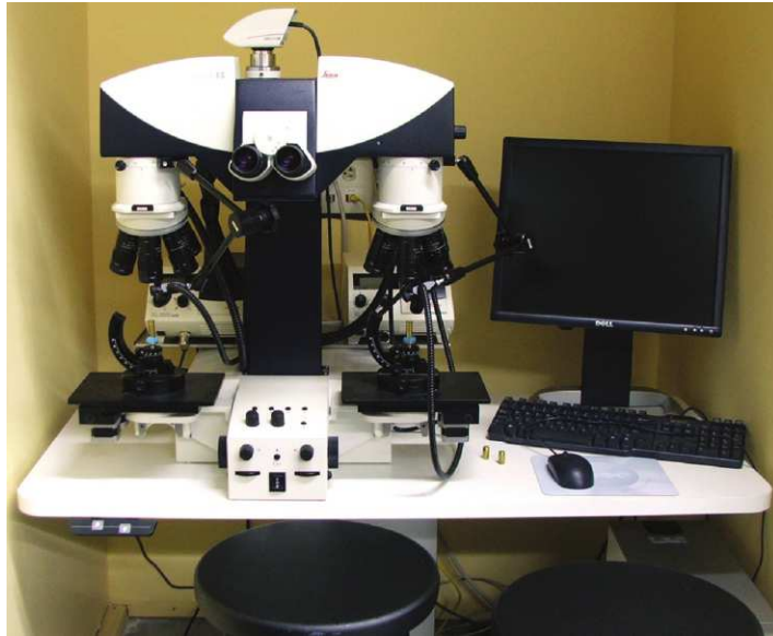
Figure 1.5 Comparison scope. This is the type of instrument used by firearms examiners today using methods pioneered by Goddard.
