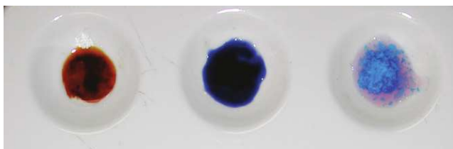
Figure 11.6 Positive color tests for methamphetamine, oxycodone, and cocaine (left to right).
