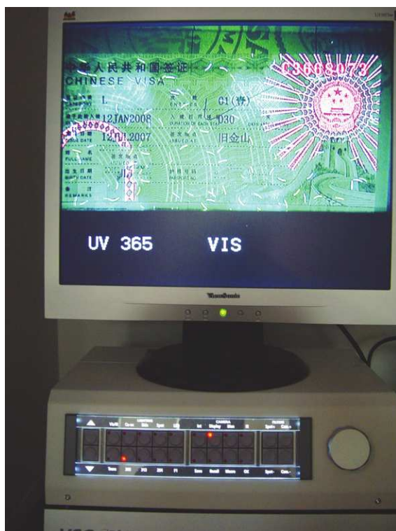
Figure 17.3 Video spectral comparator (VSC) revealing security features using ultraviolet light.
