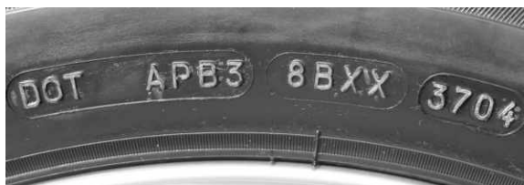
Figure 15.16 The Department of Transportation (DOT) number includes information that tells where and when that tire was manufactured.
