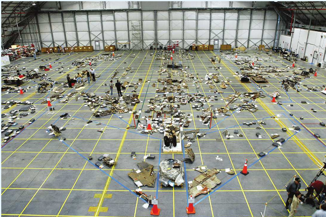
Figure CS18.1.1 Forensic engineering was used to reconstruct the Columbia accident.
