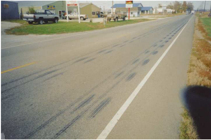
Figure 18.4 Skipping truck skid marks are usually the result of light trailer load or when trailer brakes alone are used. Measure the whole length; do not omit “skips.”
