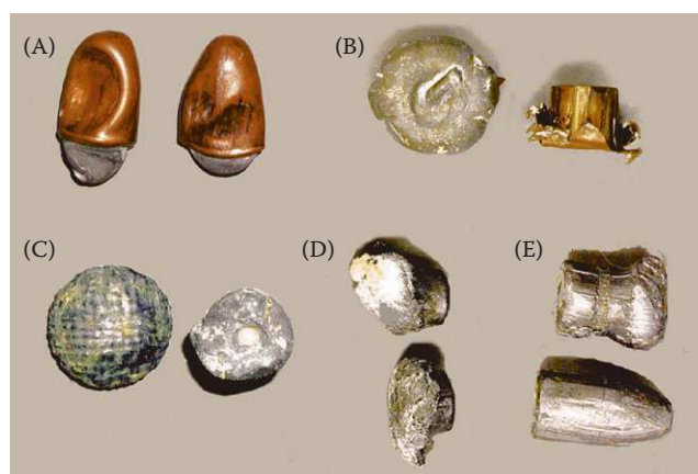
Figure 14.4 Expended bullets that might be submitted for firearms examination. (A) Deformed full metal jacket bullets. (B) Core and detached jacket of hollow-point semijacketed bullet. (C) Lead-alloy bullet that struck body armor. (D) Lead-alloy bullet that passed through window (note embedded glass particles). (F) Lead-alloy bullets that passed through plywood (note embedded wood fibers).
