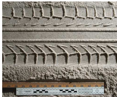
Figure 15.13 This examination-quality photograph of a tire impression depicts the tire tread design. The photograph, taken with a scale placed on the same level as the bottom of the impression, can be enlarged to natural size and compared with the suspect tire and tire impression exemplars from the suspect tire.
