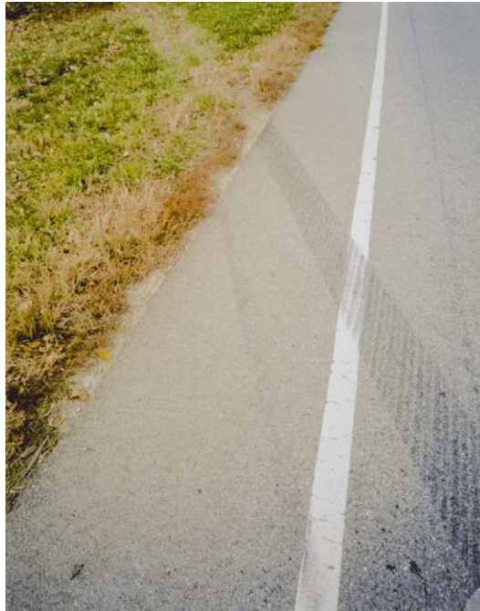
Figure 18.1 Skid marks at accident scene. Barber pole pattern in skid mark indicates tire was rolling forward at same time it was skidding sideways.
