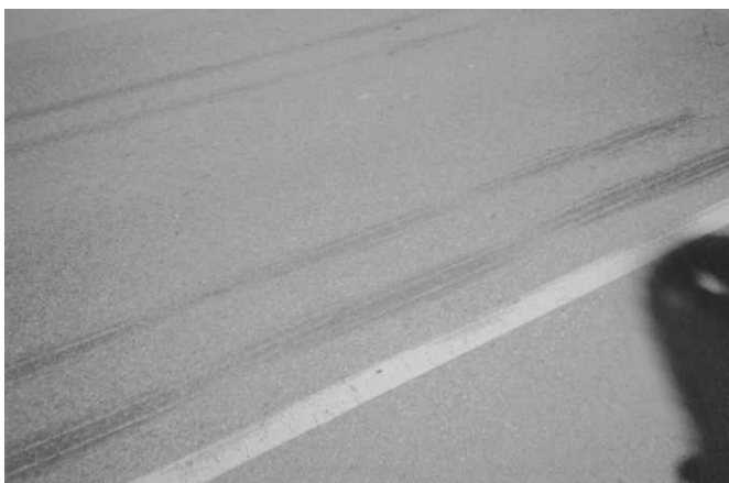
Figure 18.3 Typical truck “duals” skid mark. Straight lines in skid marks indicate tires not rotating much, or rotating and skidding in the same forward direction.
