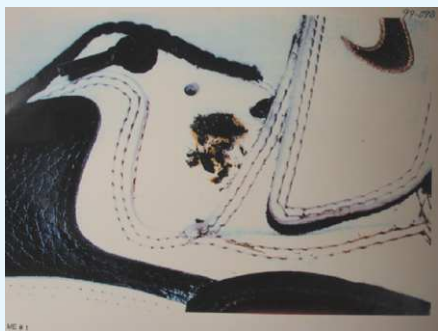
Figure CS5.1.3 Arc electric burns on tennis shoe of child who sustained electrical burns.
