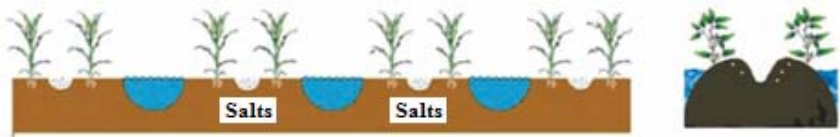
Fig. 3.8 Salt accumulation in double row planting (left) and in furrow top with a notch (right) when each furrow is irrigated
