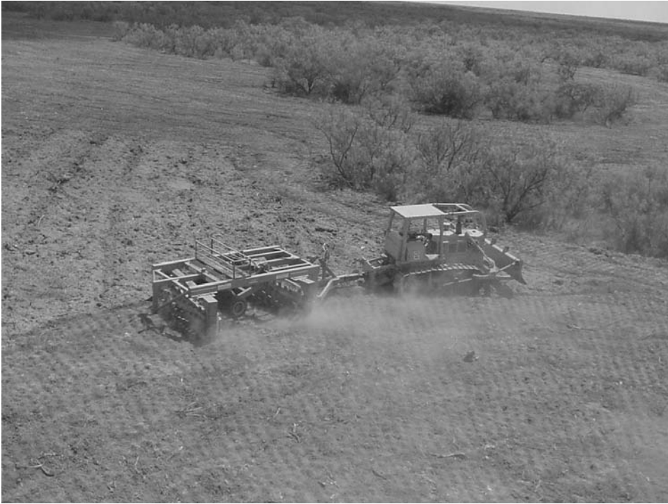
FIGURE 2.5 A roller-chopping operation being conducted on the western Rio Grande Plains of South Texas to improve bobwhite quail and white-tailed deer habitat. Roller-chopping is removing thorn scrub to restore herbaceous habitat conditions that will benefit grassland bird species (Photograph Copyright David G. Hewitt).
