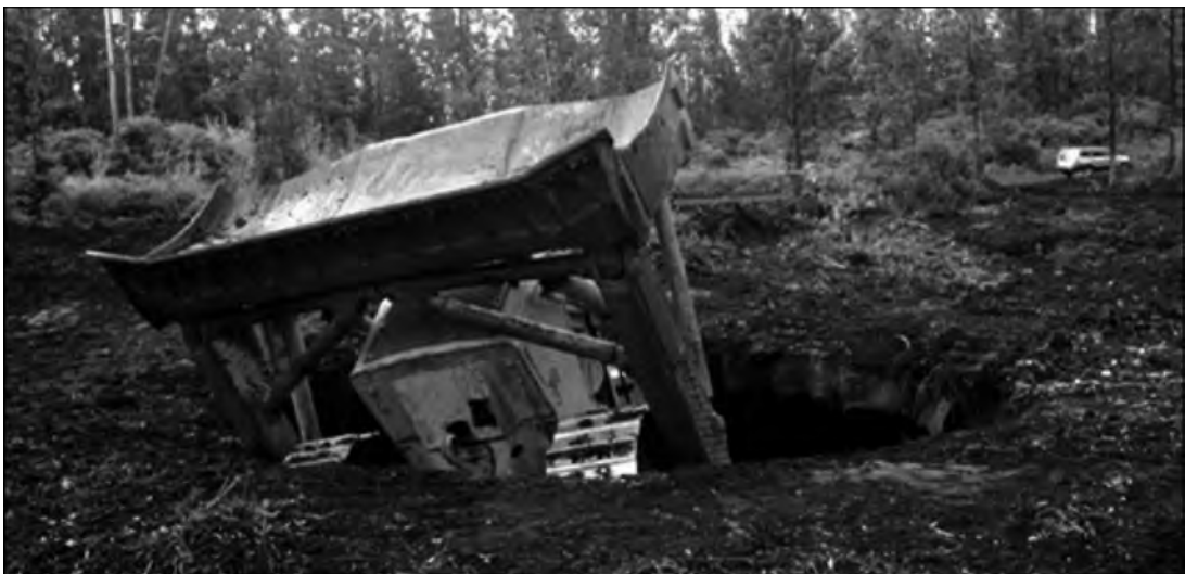
Figure 4.2 A bulldozer unknowingly clearing land above a lava tube on the Big Island breaks through the roof and falls into the lava tube
