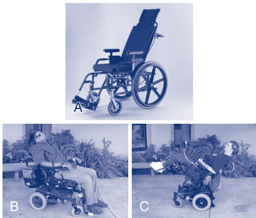
FIGURE 2-8 Manual recline versus power recline wheelchair. A , Reclining back on folding frame. B , Low-shear power recline with collar mount chin control on electric wheelchair. C , Tilt system with head control on electric wheelchair. ( A , Courtesy Quickie Designs, Fresno, Calif; B and C , courtesy Luis Gonzalez.)
