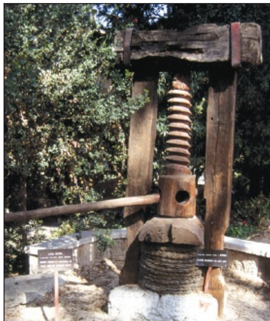
© Dr. James C. Martin Wooden screw press used to extract oil from olives.
