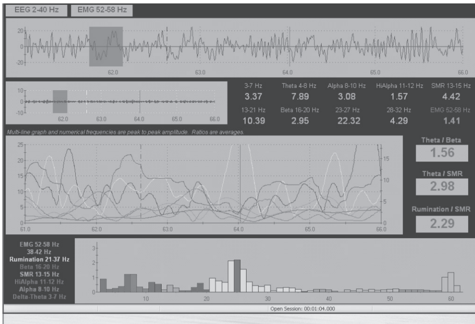
FIGURE 9.11. Spectral array at the bottom graphs power (Y-axis) by frequency (X-axis) 3 Hz–61 Hz. This client presented with anxiety and panic. Beta spindles are seen in the above figure at around 64 seconds (frequency of 25 Hz seen in the spectral array at the bottom) and at 65.5 seconds (frequency of 20 Hz).
