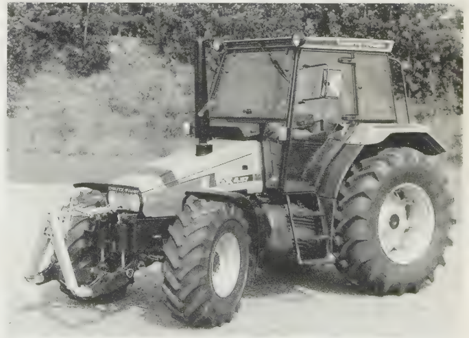
Fig. 1.8 The Deutz-Fahr DX 4.57 shown with Accord type front pick-up hitch has an engine of 66 kW (90 hp) and general design features that make it well suited to combined front-and-rear grass harvesting work, front handling operations and fairly high road speeds in many European countries.
