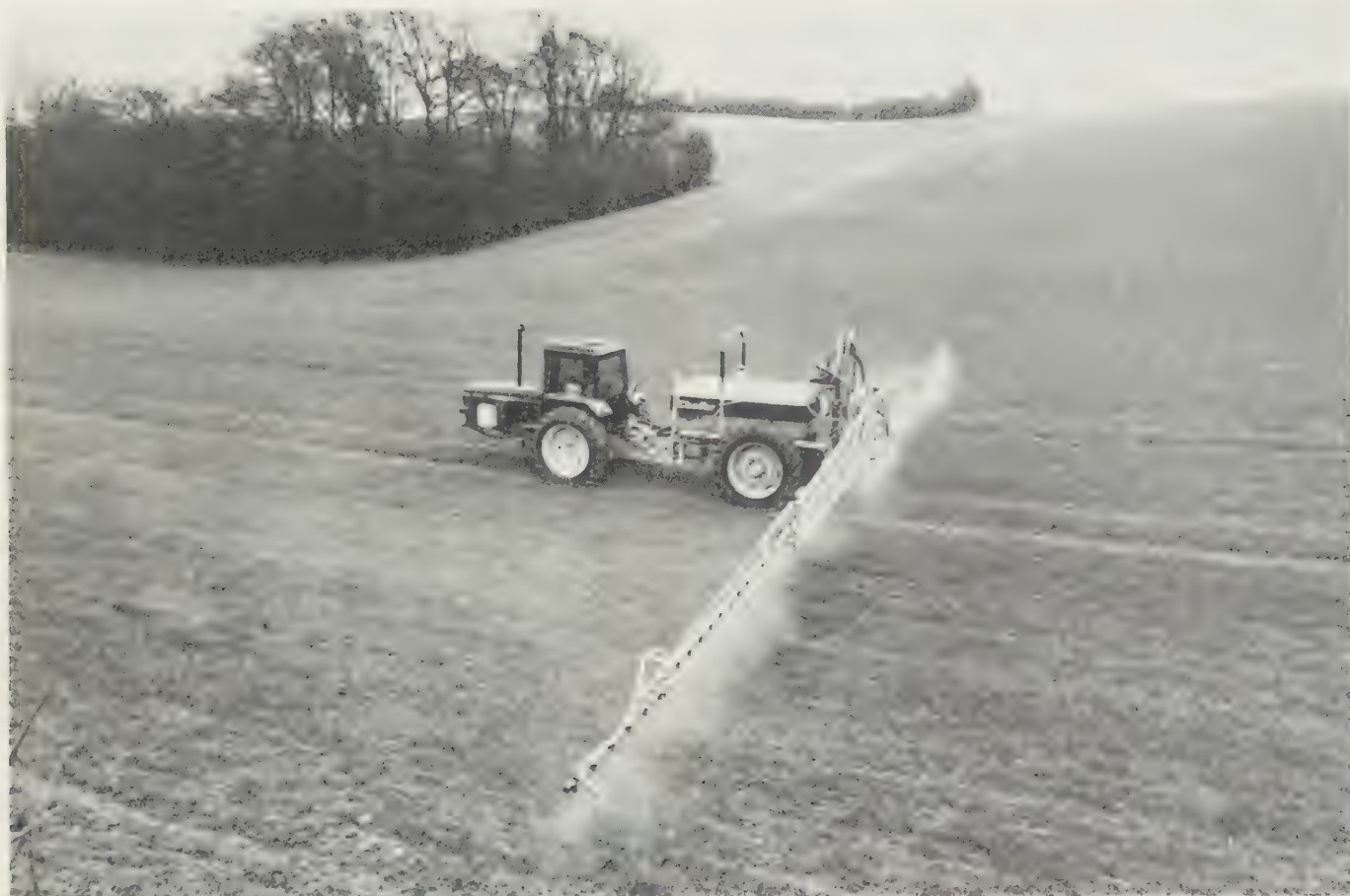
Fig. 8.8 This self-propelled 'Tramliner' high-capacity sprayer with 24 m boom of advanced design can be equipped with closely spaced 'stream' jets for nitrogen top dressings. The
