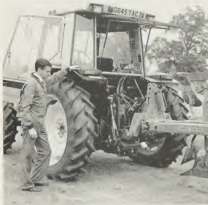
Fig. 1.10 Developments in electro-hydraulic controls have greatly improved the speed and safety of hitching heavy implements. The external hydraulic control buttons enable the driver to locate height of lift arms accurately from a safe position. (Massey-Ferguson 'Datatronic')
