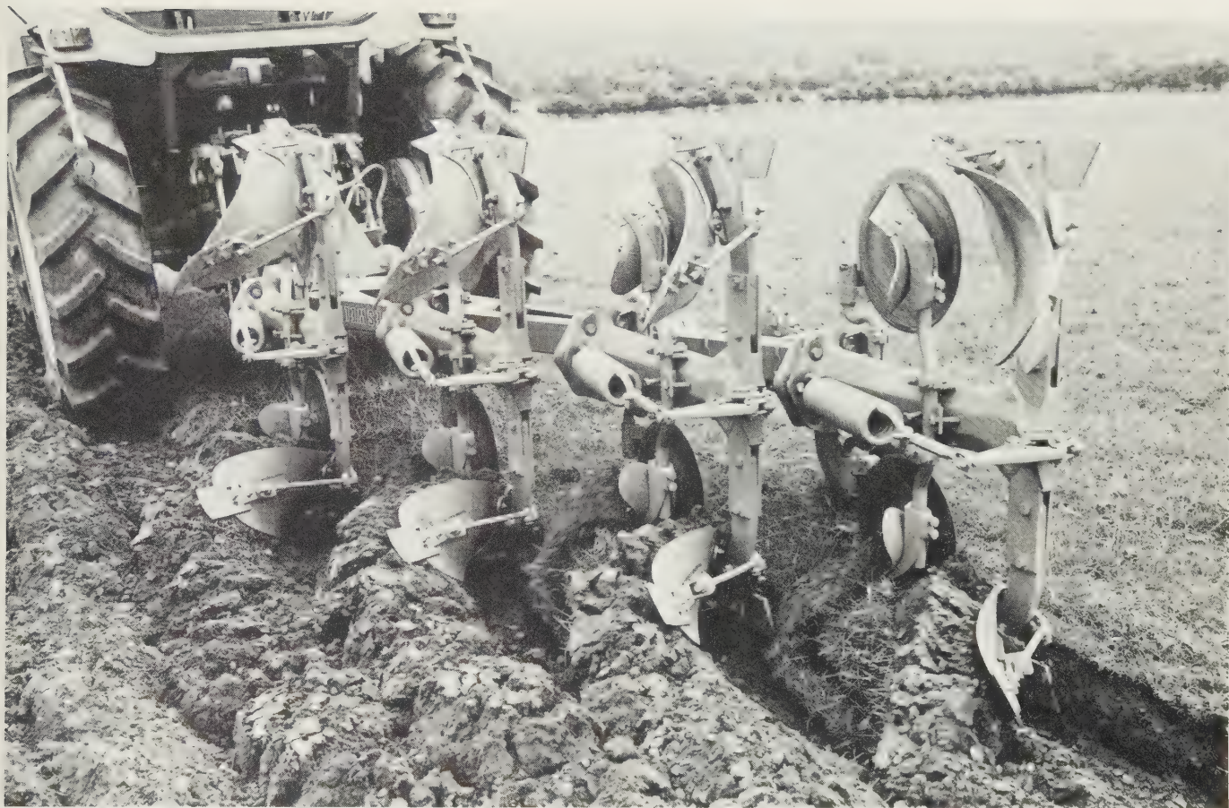
Fig. 4.7 Effective turf burial by well set skim coulters is well illustrated on 4-furrow reversible plough with auto-reset bodies. (Dowdeswell)
