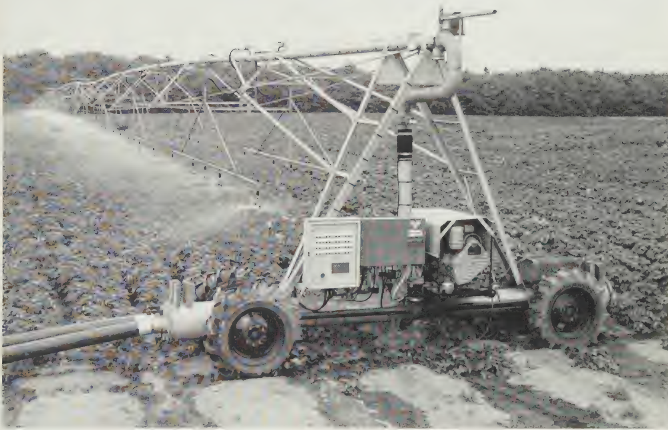
Fig. 10.14 Field-scale linear irrigation unit with flexible hose connections working in potatoes at Gleadthorpe Experimental Husbandry Farm. ( Rand/Valmont )
