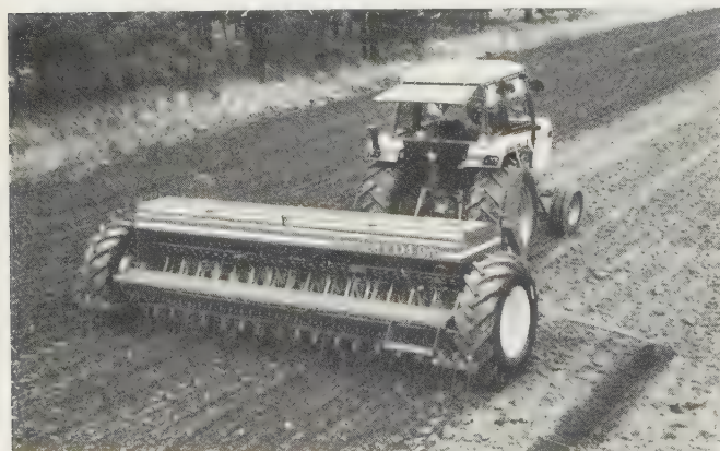
Fig. 8.10 A 4 m combine drill with 32 closely spaced coulters and direct-attached spring-tine coverers. The optional 24 coulters at 'conventional' spacing can suit heavy land better. (Richard Weston Bamlett)
