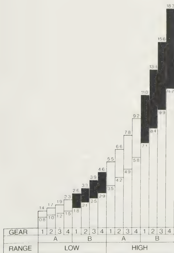
Fig. 1.4 Graph showing maximum torque to maximum speed mile/h for tractor of recent design (MF 3080) with 16-speed gearbox on 16.9/14-38 tyres. ( Massey-Ferguson )
