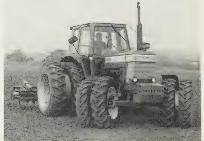
Fig. 2.12 Twin heavy-duty dual wheels for high-powered tractors are fastened together by adjustable-length hooks and eyes, using over-centre levers. Spacer steel bands secure best performance in difficult conditions. (OPICO)
