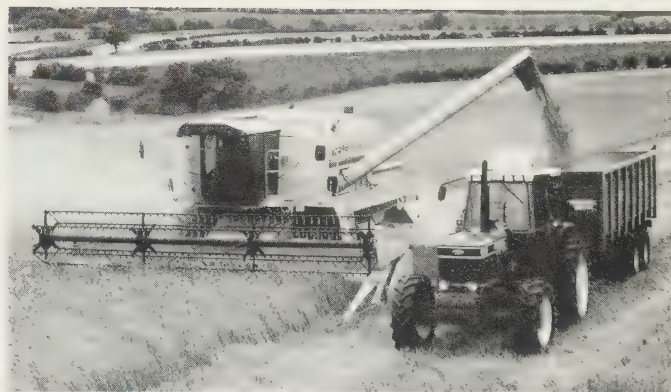
Fig. 14.17 Grain emptying on the move, using tandem axle tipping trailer. (Ford New Holland photo)
