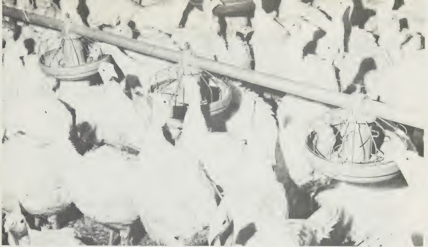
Fig. 19.17 Line of winch-suspended automatic feeders. (EB) Each line is supplied with automatically pre-weighed quantities at pre-set intervals.
