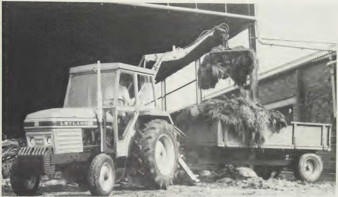
Fig. 8.14 The tractor-mounted multi-purpose slew loader can be used for loading silage or manure without unhitching. (McConnel)
