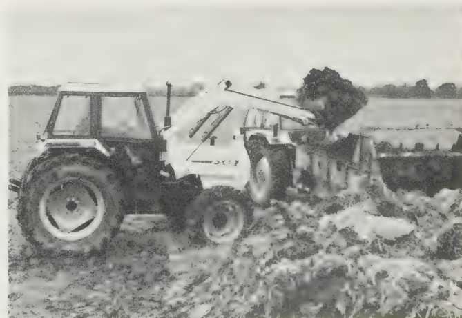
Fig. 8.12 Front loader with manure bucket on four-wheel-drive tractor loading trailer spreader. (Case-International)
