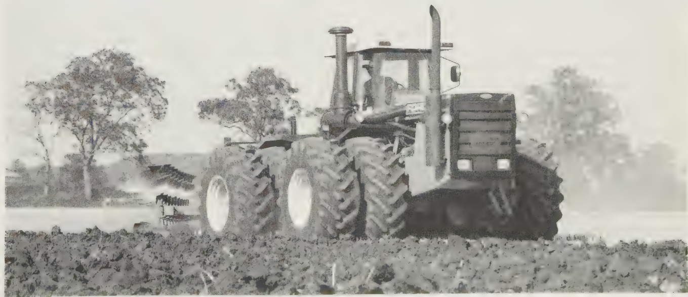
Fig. 1.9 The eight-wheel-drive articulated tractor of 300 hp is seen ploughing with Dowdeswell 10-furrow reversible plough in UK conditions. ( Ford-New Holland Versatile )
