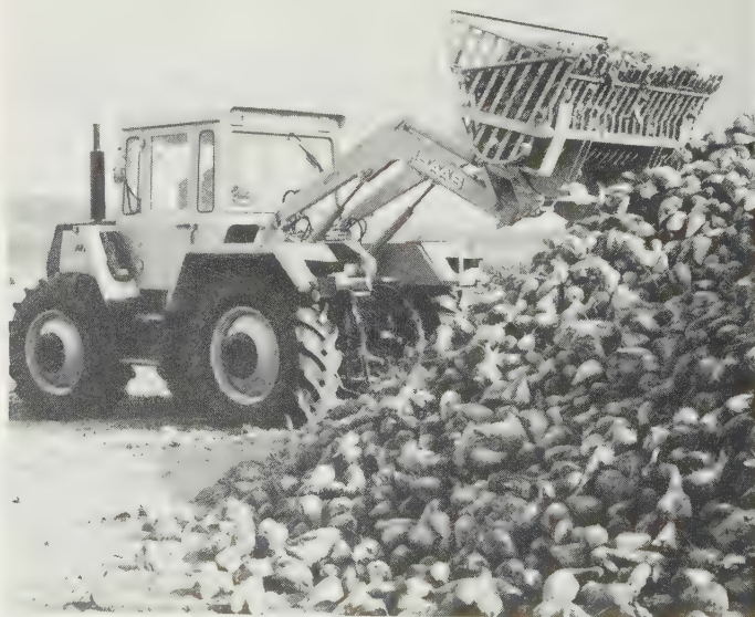
Fig. 21.11 A four-wheel-drive tractor with reverse console operating heavy-duty loader with root cleaning bucket. Mounting of loader above load platform provides good visibility. (MB-trac/Baas)
