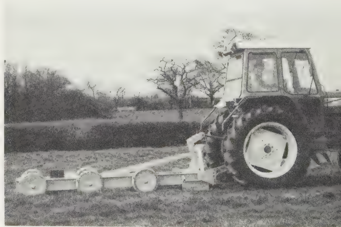
Fig. 22.11 A three-point-linkage-attached beam type mole plough with variable-pitch headstock to provide quick entry; earth-levelling skids at the front to remove clods or smooth out back-fill ridges; and three pairs of steel wheels (with scrapers) to reduce draught and secure uniform working depth. Blade pitch adjustment is incorporated; ceramic expander optional. Usual power requirement is from 70 hp. ( Michael Moore )
