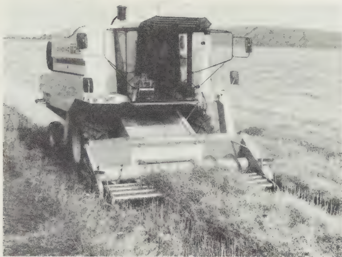
Fig. 14.3 Draper type windrow pick-up on combine with 'twin-flow' rotary grain separation, working in rape. (Shelbourne Reynolds)
