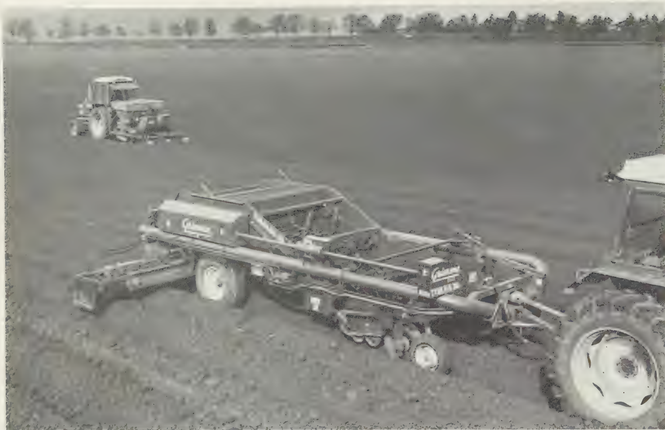
Fig. 7.24 Stone/clod separator working ahead of two-row planter. As seen here, clods are conveyed forward to furrows prepared by bed-former, which on heavy soils can set up the beds in autumn. Tractor wheels run over the clods/stones on the next bout, and the planter tractor wheels follow along the same rows. (Pearson/Grimme)
