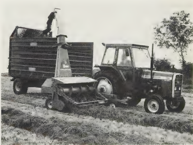
Fig. 12.2 Side-mounted ‘crop-chop’ forage harvester picking up a wilted swath is well suited to gradient work. The 24-blade chopping cylinder, directly pto driven from a right-angle drive gearbox, mounted on the three-point linkage attachment frame, moves upwards over the shear plate, throwing the crop directly up the delivery chute. The chute folds forward for easy access to the rotor. The trailer is directly ring hitched to the tractor pick-up hook. Height of the machine pick-up is regulated by vertical adjustment of the machine’s front wheel. (Kidd Crop-Chop M)
