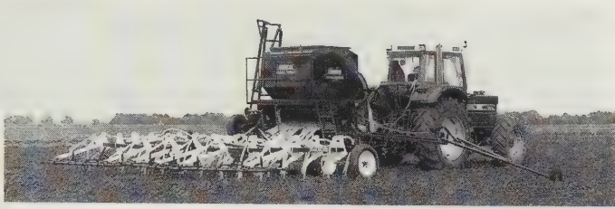
Fig. 7.7 9 metre pneumatic seed delivery cultivator drill designed for high-speed combined cultivation and sowing in UK conditions. An adjustable spring-steel comb assists seed cover when working conditions require it. ( Reco-Wil-Rich )
