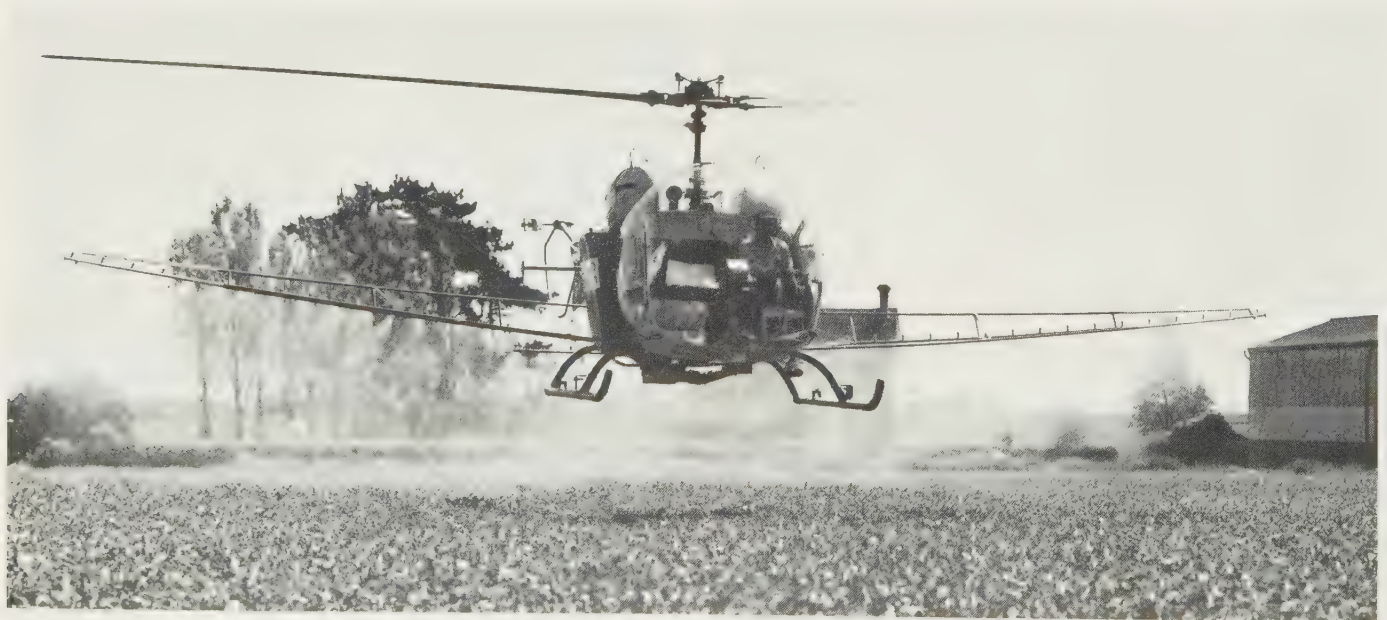
Fig. 9.20 The helicopter can spray effectively in situations where trees and buildings make operation difficult for fixed-wing aircraft. ( National Association of Agricultural Contractors )
