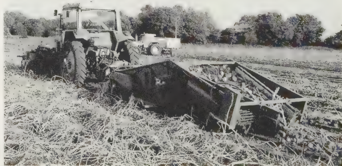
Fig. 15.2 Stage 1 of windrow harvesting potatoes in Eastern England. A heavy growth of tough previously sprayed haulm is being treated by a front-linkage mounted hydraulically powered two-row Standen flail toppler which incorporates a side conveyor belt to deliver the chopped haulm into the tractor wheel marks. The two-row potato windrower leaves the crop in narrow windrows which after a few hours drying can be picked up fast by a two-row unmanned side-loading harvester which has its intake suitably narrowed and adjusted to a shallow depth and gentle slope. ( Standen Windrower )
