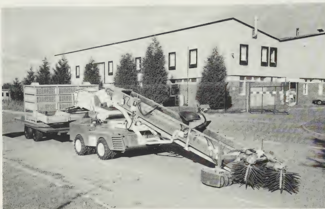
Fig. 19.19 Automatic chicken catcher. Comprising catching unit, chassis truck and crates loading system: made by Agritec under British patent licence from British Technology Group.
