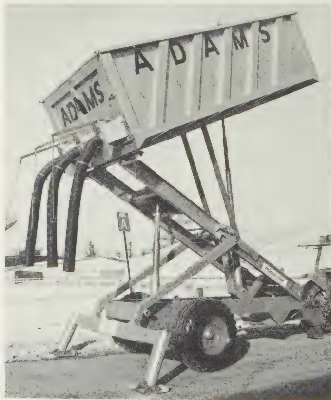
Fig. 21.3 Safe high-tip trailer with stabilising legs, hopper divisions and controls for fast easy filling of drills with seed and fertiliser. The tractor may be unhitched and the trailer left tipped. Auxiliary oil reservoir and controls on trailer are used to avoid lowering tractor oil level. (Adams Wagons)
