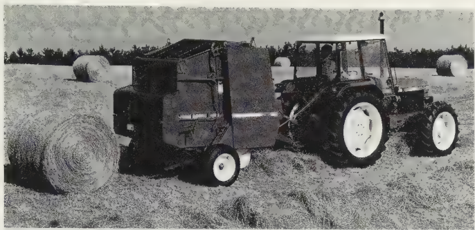
Fig. 13.15 Second generation machine of variable diameter rough-surface endless belts type can produce uniformly dense hay or higher-dry-matter silage bales at high speed with electronic in-cab control of all operations including net wrapping. Illustration shows part of range of bale diameters with net wrap. Width is 1220 mm (4 ft). (John Deere 545)
