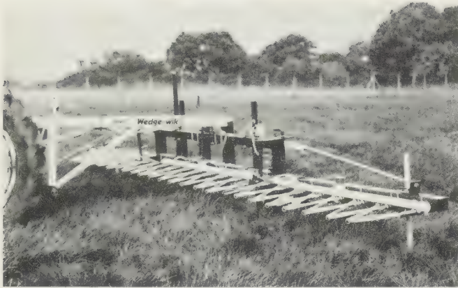
Fig. 9.19 Rear-mounted herbicide wick-on applicator with wedge arrangement of wicks and pressure regulated spray supply system. Each V-section is fed via a stainless steel metering tube; flow rate can be varied from cab to suit weed infestation density. ( Vicon 'Wedge-Wik' )
