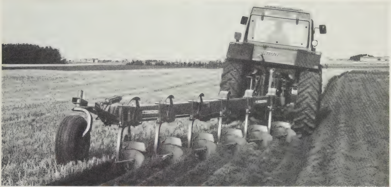
Fig. 4.5 Method of plough construction with single diagonal beam and parallel action furrow width adjustment allowing easy change of furrow width on the go. Bodies fitted with trashboards above and ahead of mouldboards help to bury stubble completely. (Kverneland)
