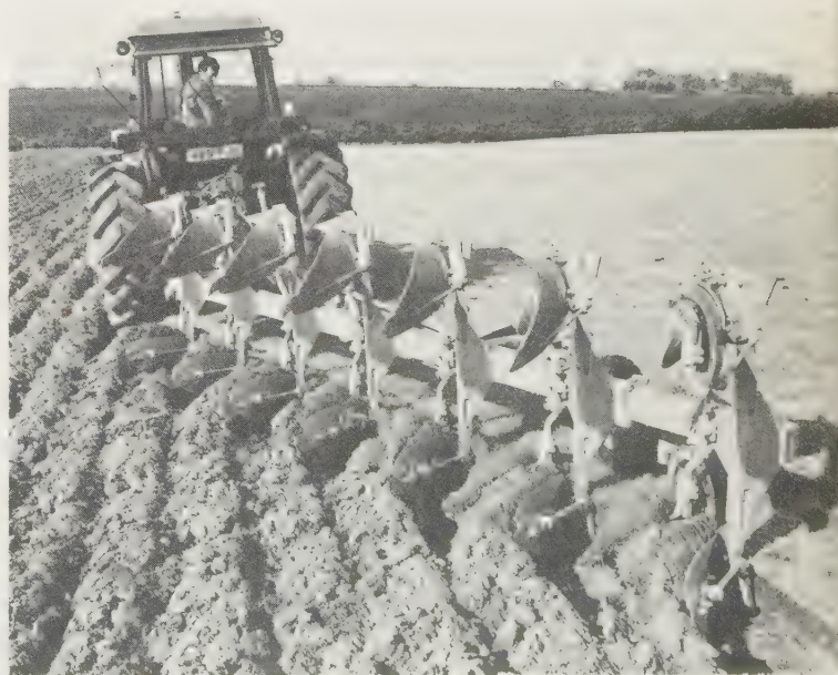
Fig. 5.2 A 7-furrow fully mounted plough with headstock adapted to US Category 3 Quick-Hitch on 190 hp four-wheel-drive tractor. With well set skimmers the turf is effectively buried. (Dowdeswell)
