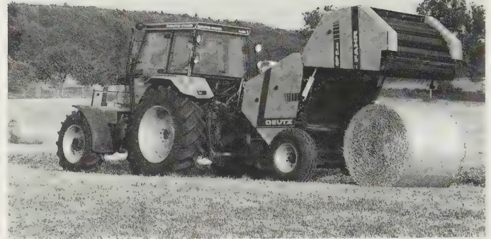
Fig. 13.19 This fixed-chamber-size machine produces bales of 1.2 \times 1.2 m ( 4 \times 4 ft). As with multi-purpose machines of similar type, net wrapping has the worthwhile advantages of tidy bales and a considerable saving of time compared with use of twine. It can maintain a consistent bale density over a range suited to straw, hay and wilted silage. (Watveare/Deutz-Fahr)
