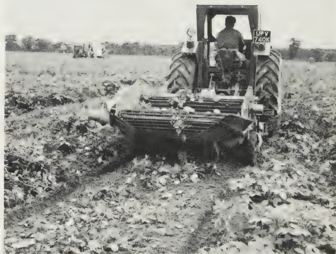
Fig. 15.1 Semi-mounted two-row elevator digger fitted with belt-type chain for lifting an early crop. Mid-mounted castor wheels facilitate short turns. (Blair Engineering/Ransomes)
