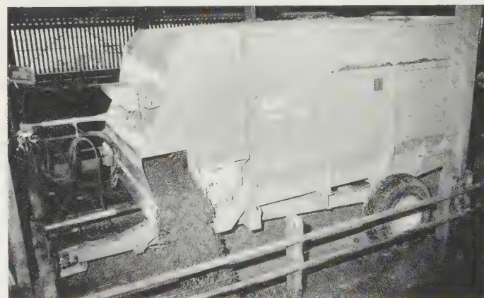
Fig. 12.20 Largest of range of mixer-feeders designed for handling mixes of straw, silage, concentrates and brewers' grains, but equipment also available for chopping fodder roots if required. Capacity is 11 m 3 (14.4 yd 3 ). Extra-heavy-duty chassis: fodder mixed and shortened by three horizontal tined beaters in a vertical row across the front of the box. Main floor conveyor is hydraulic drive full-width rubber belt that normally moves forward towards the beaters on a bed of rollers, taking the load in a coherent block at a slow speed, infinitely variable, to the beaters. Discharge by variable speed hydraulically driven rubber belt disc to either side, and floor belt is reversible if needed. Concentrate dispenser and weighing equipment optional. Layering the feeds at loading is not unusual. Power requirement 12 kW (15 hp). Suitable for large herds and sometimes two herds. (Kidd 400 XC)
