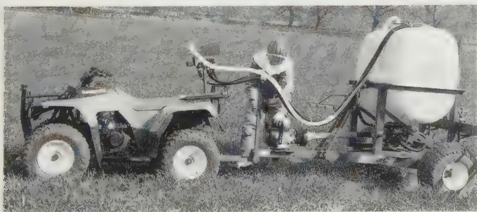
Fig. 2.41(b) Four-wheel-drive ATV with engine driven 600 l capacity sprayer on two-wheeled chassis carrying 12 m spray boom. ( Kawasaki/Logic/Allman 'Cropguard' )
