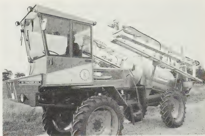
Fig. 9.13 High-clearance self-propelled sprayer/spreader with articulated 'tracker' chassis and mechanical four-wheel-drive equipped with 85.5 kW (120 hp) engine, 2500 litre spray tank and 'Alulight' boom. The multi-purpose chassis is designed for easy removal of the sprayer unit and replacement by fertiliser spreader or pneumatic drill unit. Engine size range is up to 134 kW ( Turbo ). Tyres shown give 940 mm axle clearance; LGP tyres for soft wet soil conditions available. 5 × 2 Synchromesh gearbox gives ten forward and two reverse speeds. Independently variable-speed pto drives sprayer pump or distributor. Spray automatic control by RDS Rate Master. Cab provides air suspension seat, tinted glass and full air conditioning with carbon filtration. ( Willmot Hi-Tracker 2514 )
