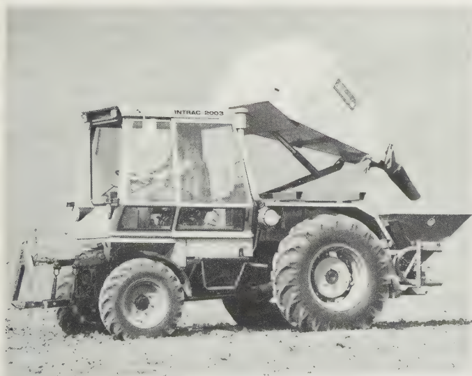
Fig. 21.5 The hydraulically operated bulk hopper can replenish the fertiliser distributor on the move. (Deutz/Hassia)
