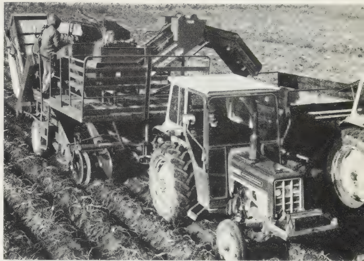
Fig. 15.4 Offset single-row harvester with stone separator attachment (brush type) and picking-off platform. Machine is shown opening out, using trailer-loading elevator. (Pearson/Grimme 'Row-over')
