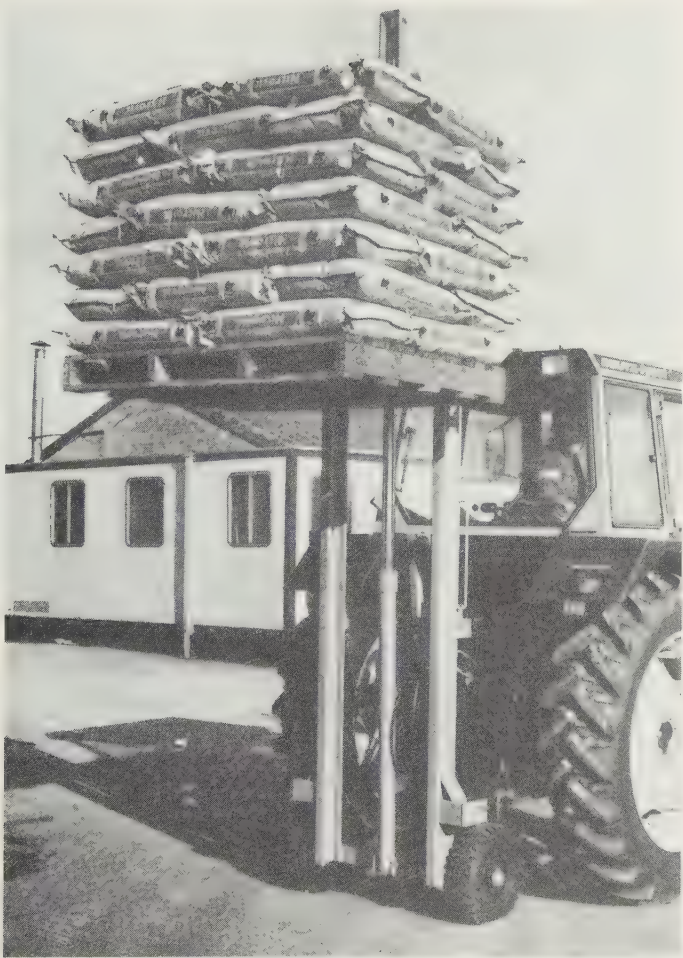
Fig. 21.12 Wheel-supported linkage-mounted tractor fork-lift with 2 tonne load capacity. ( McConnel Ripvator )
