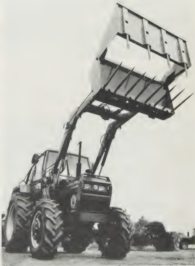
Fig. 21.13 'Triple' Front Loader attachment with in-cab operated hydraulic folding of the hinged upper member to change the purpose from long-tine-fork, via fork with retaining grab for soft fluffy materials, to large-capacity bucket for soil, sand or ballast, and vice versa. ( Portec UK )
