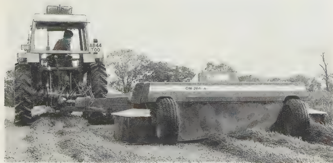
Fig. 11.5 High-capacity four-drum rotary mower with two large-diameter outer drums rotating inwards and two smaller diameter inner drums rotating outwards, initially forms two swaths which may be moved alongside one another by two adjustable rotary swath formers if required. The mower in work is attached to the drive at a wide angle which can be reduced while mowing by use of in-cab finger-operated hydraulic control. This makes it easy to avoid obstacles, take less than the maximum 2650 mm cutting width or move completely out of crop prior to folding end guards and raising for road transport. For measurements see text. (SKH/PZ (Zweegers) CM265A)
