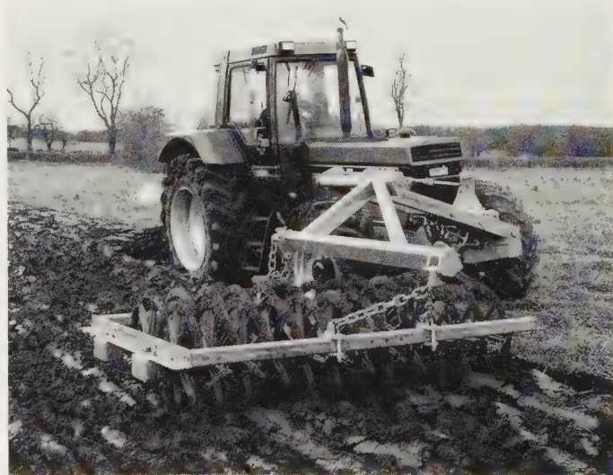
Fig. 3.1 Double-row front-mounted swing-over furrow press used in conjunction with well-set large skimmers on a matching reversible plough provides effective non-stop seedbed preparation in a single pass where a mat of surface trash needs to be buried. The hydraulically operated centrally pivoted front-mounted press is attached by heavy-duty brackets to both sides of the tractor frame and helps to balance the weight of the reversible plough on headland turns, and when being moved along roads. (Dowdeswell)
