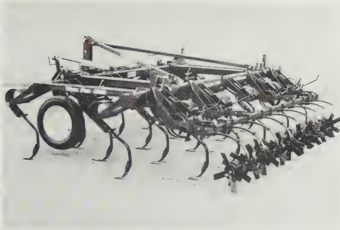
Fig. 6.4 Mounted cultivator-harrow for high-speed work with four rows of flat-spring-top tines designed for intense vibrating action and Rotoflex attachment for straw breakdown and mixing. (Kongskilde 'Vibraflex')
