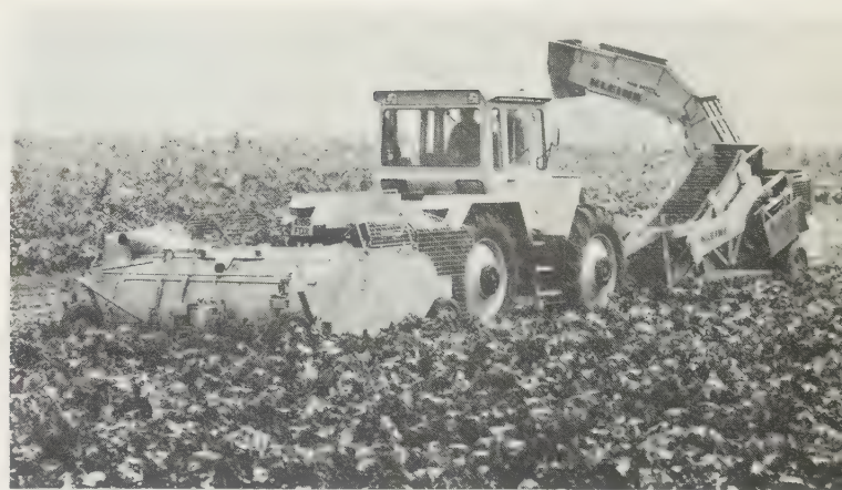
Fig. 15.23 Tractor having reverse console used front-to-rear with six-row beet topper-lifter and windrow pick-up loader. ( Kleine on M-B-trac )
