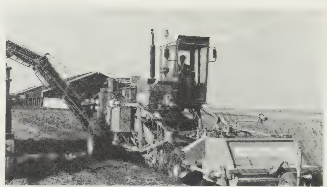
Fig. 15.7 A two-row self-propelled side-loading multi-purpose potato, vegetable root crop and bulb harvester. The 70 kW hydrostatic drive power frame has drive wheels of adjustable track width and is shown with front-mounted topper. Other optional attachments include onion windrower. (Amac)
