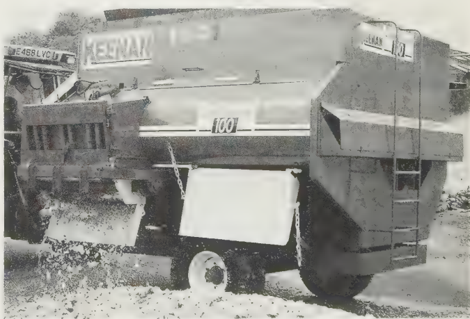
Fig. 12.21 Large capacity complete diet feeder with option of built-in chopper for root crops such as fodder beet to give cleanliness and consistency suitable for mixing with other forages, straights and by-products to produce economic diets. (Keenan Combi-feeder 100)
