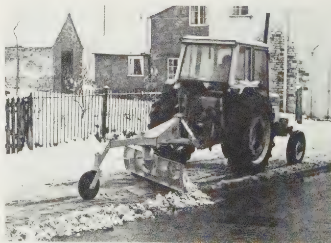
Fig. 22.13 General-purpose grader/scrapper with easy adjustment of blade angle, blade tilt and beam offset demonstrates its versatility. (Bomford)
