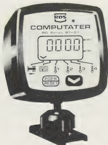
Fig. 7.20 Potato planter monitor as mounted in tractor cab, for finger-tip operation. The monitor is normally operated with forward speed displayed, as indicated by the small black chevron above the extreme left channel. Moves to other channels are by pressing the white chevron in black surround (see text). (RDS 'Computater')
