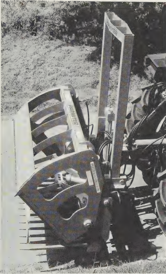
Fig. 12.16 Tractor rear mounted Shear Grab silo unloader developed for European markets with mast, push-off attachment and closely spaced tines. (Parmiter SG 250)
