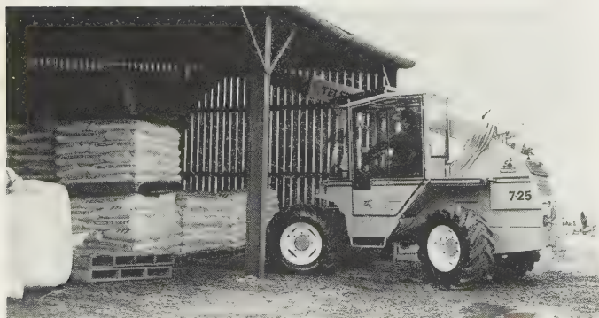
Fig. 8.5 On a large-farm scale fertiliser handling is an operation that benefits greatly from use of a handling vehicle with all-wheel steering and a telescopic boom with long reach and adequate lift capacity. For machines with a large bulk hopper, use of big bags is increasing, but pallets have advantages for high storage. Handling vehicle illustrated is the Teleporter 2 equipped with single joy-stick 'solo' boom control. (Originally made by Sanderson)
