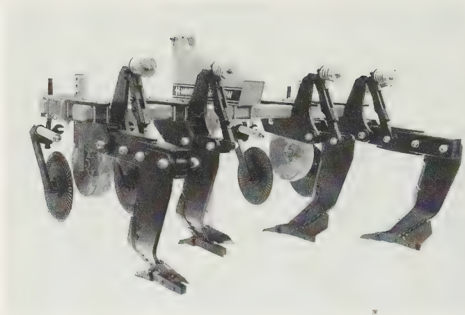
Fig. 5.11 Up-dated balanced 'Paraplow' with two right and two left-hand legs mounted on opposite sides of the sturdy mounted frame. Two depth regulation wheels are mounted just forward of the main beam. All legs have a long vertical length at the top and an automatic break-back device for stony conditions or deep work. The discs also incorporate a spring release. ( Howard-Farmhand )
