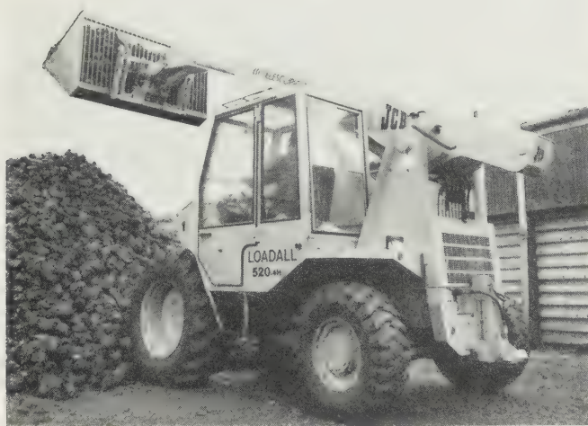
Fig. 15.24 A four-wheel-drive telescopic-boom rigid-chassis loader with grille type root bucket and pick-up hitch for trailers tidying up sugar beet clamp. (JBC)
