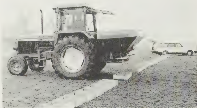
Fig. 8.1 Twin-disc fertiliser distributor undergoing manufacturer's Technical Services Division field tray test for calibration and evenness of distribution. Results are weighed and recorded in detail in the field, and later analysed and printed out in histogram form by a computer with specially designed computer programme used for controlled tests in a large purpose-built test laboratory. ( AMAZONE ZA-U twin-disc spreader )
