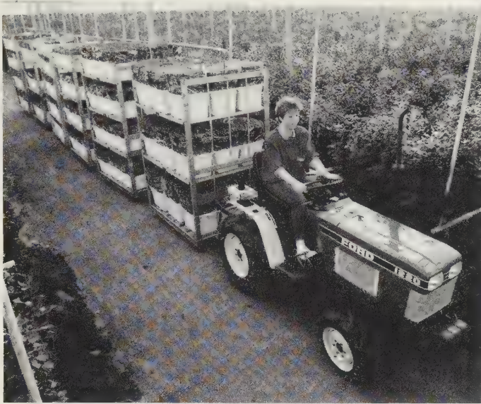
Fig. 2.46 Compact tractor (16.7 DIN hp) working in a commercial glasshouse. ( Ford New-Holland )
