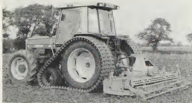
Fig. 2.44 Rubber belt half-tracks used on Massey-Ferguson 3080 for high-speed power drive seedbed preparation. (Colmant Cuvelier Kitco tracks)
