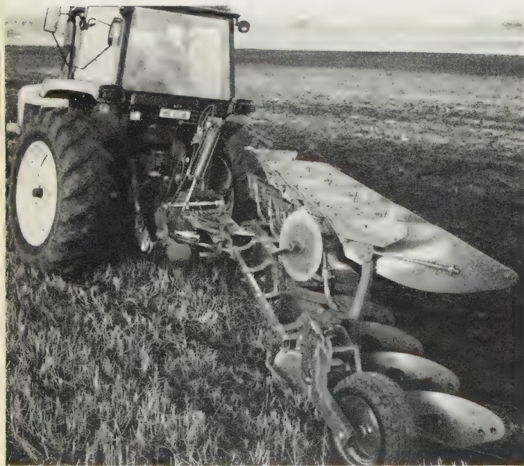
Fig. 5.1 Reversible mounted plough with single-component main beam and 5 variable-width pairs of bodies adjustable on the move from 30–50 cm (12 to 20 in) by horizontal ram just above lower hitch pins, acting through bar running parallel to main beam (See also Fig. 4.6). ( Kverneland )
