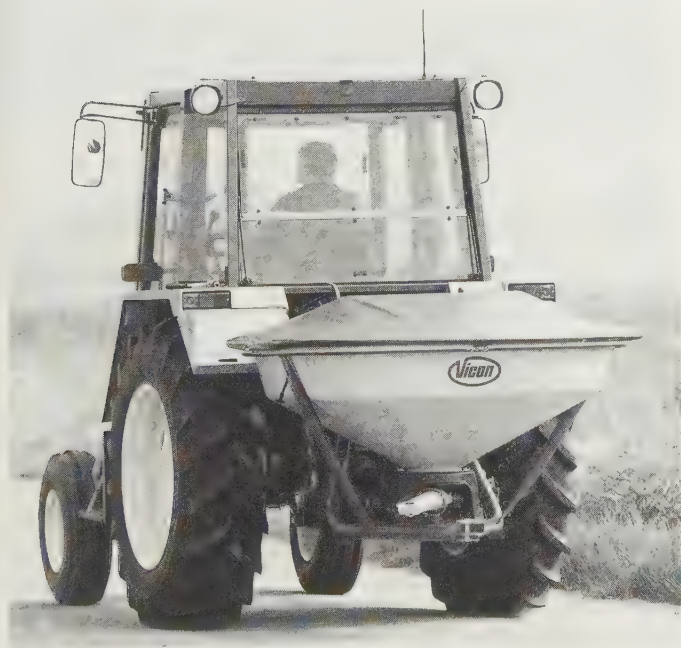
Fig. 8.2 Mounted fertiliser distributor with oscillating spout delivery. Hopper can be mounted on a high-lift frame for top-dressing at late growth stage. (Vicon Varispreader)
