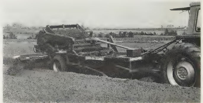
Fig. 7.23(b) Stone and clod separator with floating intake rotor and long adjustable scrubber/clod crusher web above the steeply sloping rear web. Three rows of hydraulically actuated pressure pads are located above the floating web to improve separation in damp or cloddy conditions. The machine is seen working on the deep-ridged forward burial system. ( Reekie 330 SA )
