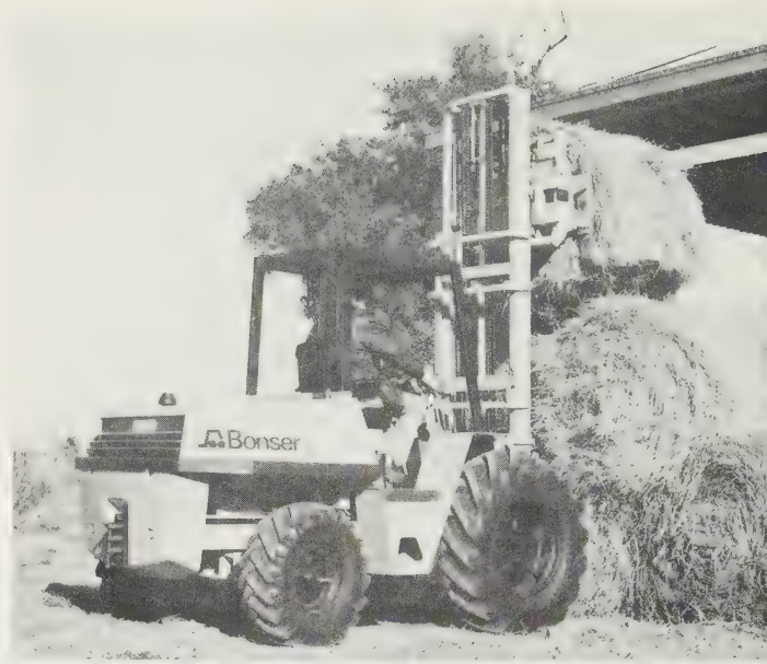
Fig. 21.14 Conventional mast-type RTFLT stacking big bales in barn. Counter-weight assists in providing stability in high-lift situations. Good operator visibility and ease of control are normal design aims. ( Bonser )
