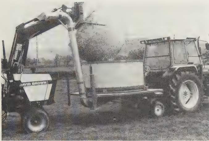
Fig. 19.23 Tractor rear mounted big-bale straw chopper with tub diameter 1.88 m (6 ft 2 in) being loaded with wrapped big bale. The tub has hydraulic drive and three possible outlets giving a choice between normal and short chop, plus an elevated 'Kobra' outlet as fitted, or flexible blower format with up to 10.7 m (35 ft) of 180 mm I.D. (7 in) plastic tube, with or without adjustable gantry facility (applies to model 6–10 only). Stabiliser wheels are fitted to top model only. (Kidd Model 6–10)
