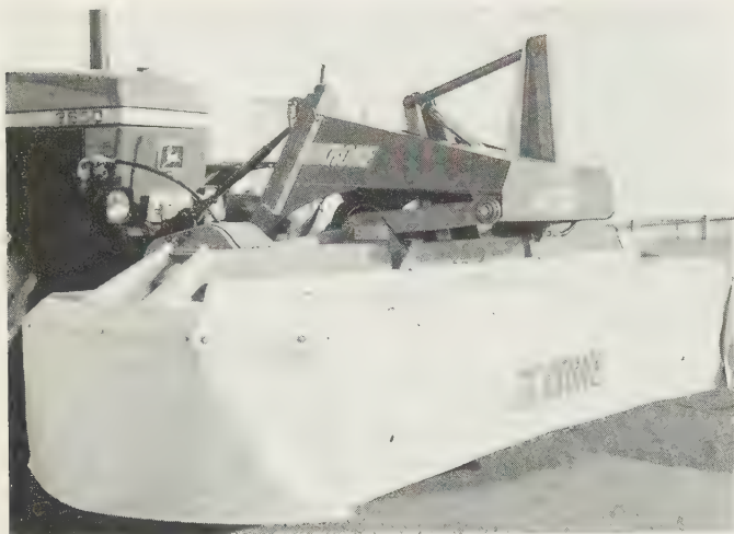
Fig. 2.31(a) Front-mounted mower-conditioner with 2.8 m working width showing rigidly attached forward extension from the front three-point linkage enabling the use of a front-hinged suspension system to provide easy float on undulating surfaces. (Krone AFL 282 Z)
