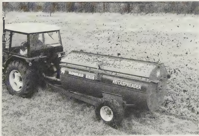
Fig. 8.19 Rotary flail side-spreader with 'original' A-frame chassis construction, capacity 4.2 m 3 (5.5 yd 3 ) (Model 1552 Howard Rotaspreader)
