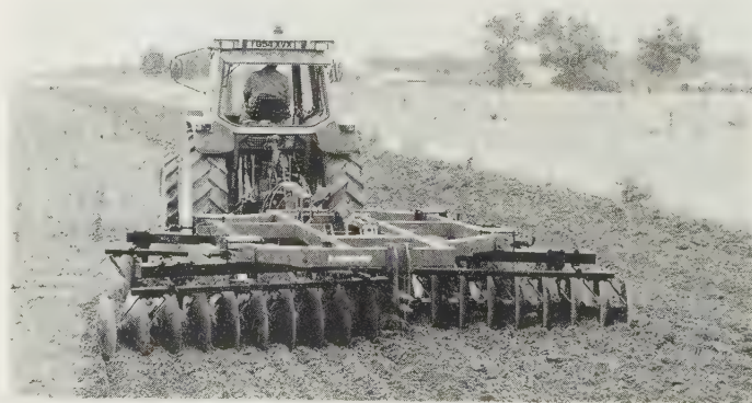
Fig. 6.11 Ransomes 'Incorporator' tandem disc harrow with hydraulic depth control/transport wheels and manual folding. ( Agrolux )
