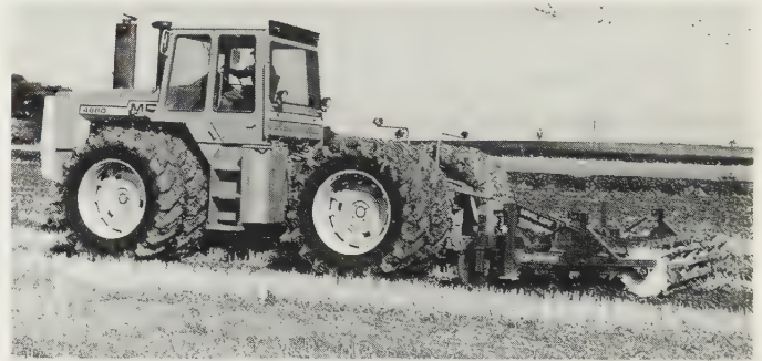
Fig. 2.36 Eight-wheel-drive tractor with articulated frame steering ( Massey-Ferguson 4880 ) seen breaking stubble with level-lift deep cultivator ( Cousins ). Centrally located pivot pins and a horizontal trunnion assembly allows a limited degree of rotation between the front and rear parts over ground undulations. Electronic lower link sensing may be employed for three-point-linkage equipment.
