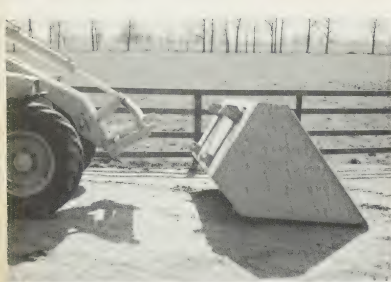
Fig. 21.19 Quick-attachment mechanism. Bucket is first raised by pair of hooks and then tilted back. Lower pins are inserted by use of hydraulic control in cab. (Sambron)
