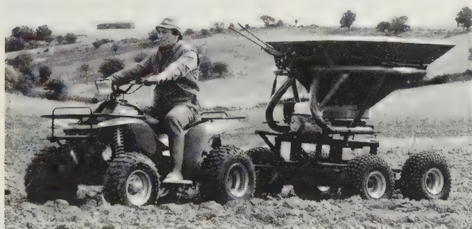
Fig. 2.41(a) Powerful 'mini-tractor' (244 cc air-cooled oil injection) with automatic variable transmission pulling four-wheel LGP vehicle equipped with engine-driven fertiliser distributor. ( Polaris Trail-Boss 4 x 4 with Logic System 40 vehicle )
