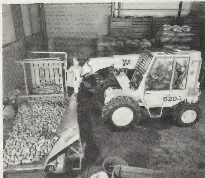
Fig. 21.20 Specialised handling capabilities of telescopic-boom vehicles can include a rotary box tippler for gently emptying potato boxes. (JCB)
