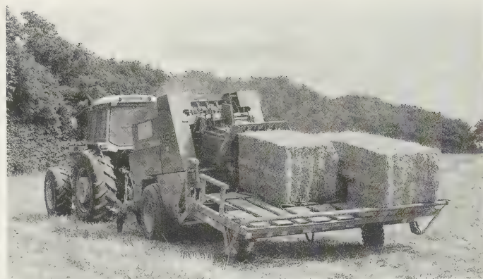
Fig. 13.9 In-line big baler delivering second bale centrally to Browns Tipper accumulator, which later moves it left to make way for third. Bale size is 0.8 by 0.8 m section and up to 2.5 m long. (Massey-Ferguson MF-5)
