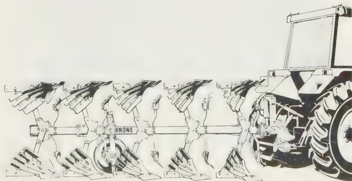
Fig. 4.3 Reversible ploughs with slatted mouldboards and reinforced chisel share points are widely used on light flinty soils in many European countries. (Krone)
