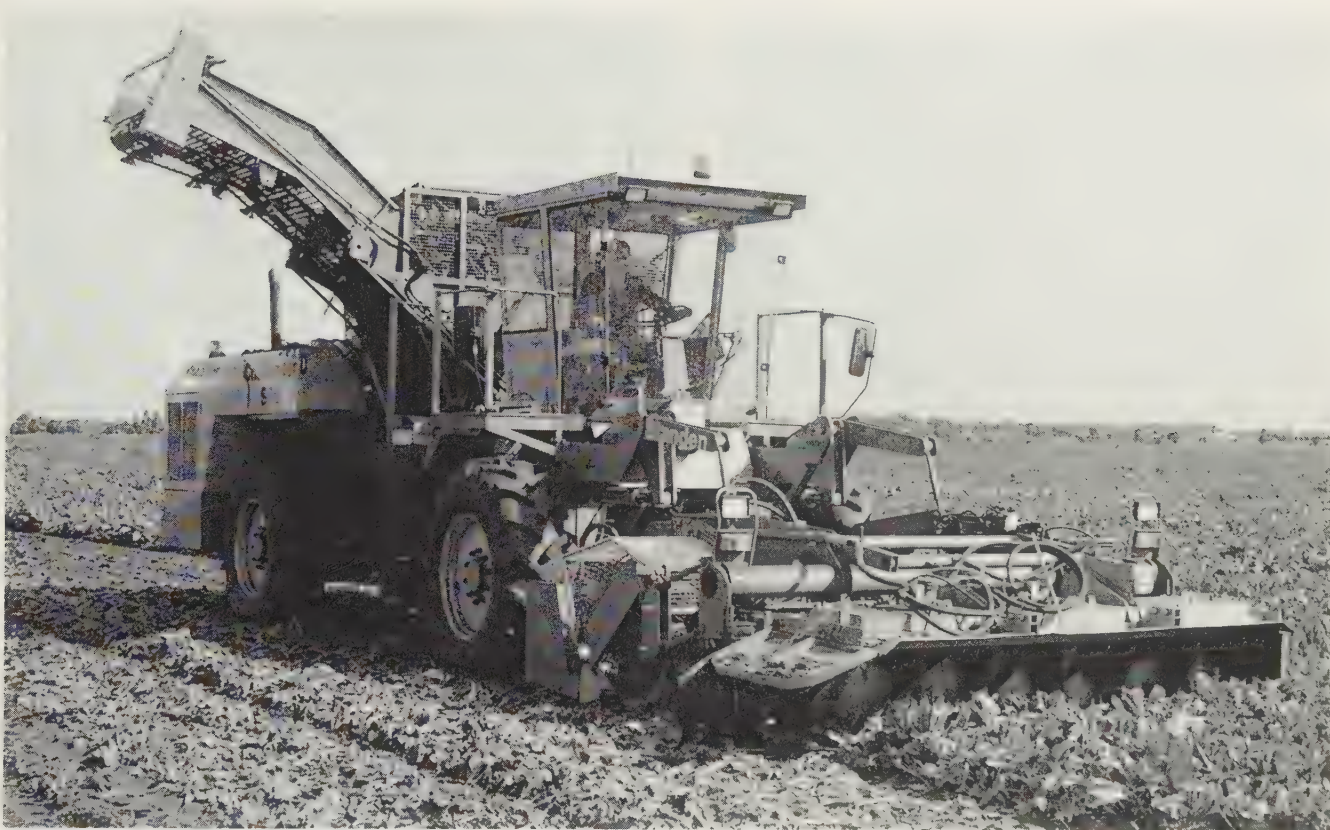
Fig. 15.17 Six-row self-propelled sugar beet harvester powered by 200 kW (268 hp) engine with four-wheel drive and four-wheel steer hydrostatic drive to equal-sized wheels. Rear wheel drive only is available for roadwork, and automatic differential lock is an option in the low gear range. Tight headland turns are provided by a manually operated 'steer assist' lever operating on the rear wheels. Ability to take mechanical drive power from both ends of the engine assists a logical distribution of the main components with the engine and its tanks well to the rear where direct mechanical power can be used for driving cleaners and elevators. Electronic sensors and microprocessor provide distance, area and forward speed information. In-cab noise level is lower and seat better than normal tractor regulation requirements. (Standen 'Challenger' SP6)
