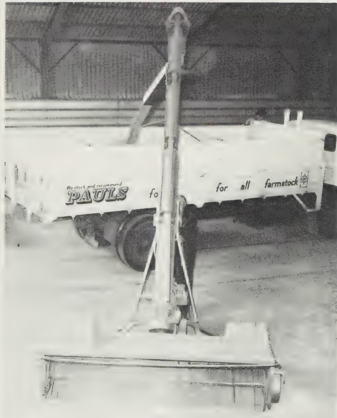
Fig. 18.24 Sweep auger used for loading grain into bulk transport vehicle. ( Ardleigh Swift )
