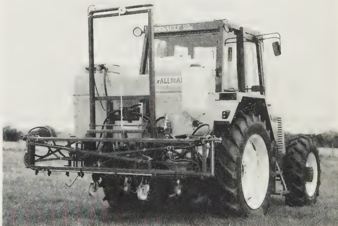
Fig. 9.1 Medium capacity model from modern tractor-rear-mounted sprayer range fitted with 12 m manually folded hydraulic raise/lower boom. (ALLMAN ACE range) Features include short and wide saddle-shape moulded tank with central strengthening tunnel providing direct run for linkage to boom and neat routing of pipes from controls to nozzles. External cylindrical chemical inductor vessel (right); and built-in clean water tank (top left). Usual control system for model suited to tractor of 52 kW (70 hp) is manually operated and incorporates automatic proportional flow regulator effective over minor speed variations in same tractor gear. Diaphragm pump located for accessibility and flooded suction: stainless steel spray lines; 110° colour coded nozzle tips in self-aligning caps at 500 mm spacing. Larger models in range incorporate electro-hydraulic boom folding, solenoid-operated boom selection valves and options for fully automatic spray regulation.
