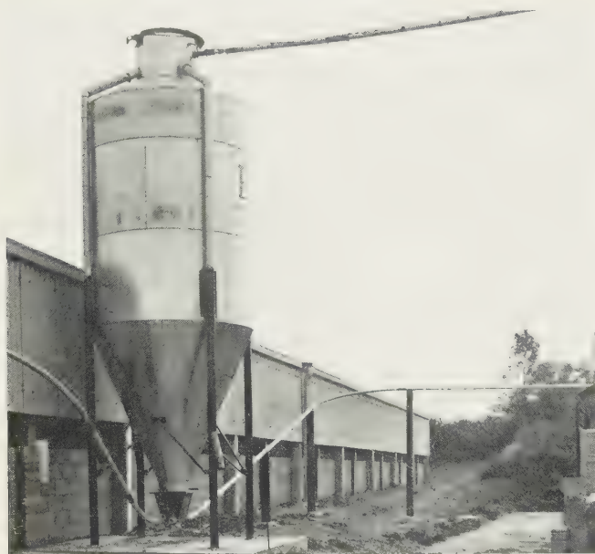
Fig. 19.3 Open-centre flexible auger used to convey concentrate from bulk hopper to dispensers in livestock buildings (EB). Distance up to 80 m (250 ft); rate up to 1 tonne/h.
