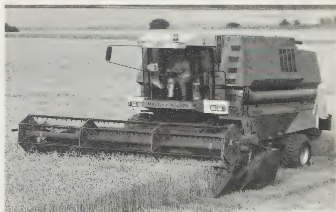
Fig. 14.6 Large-capacity 'conventional' design combine harvester of European origins with very comprehensive electronic monitoring of a wide range of functions and output performances, accompanied where helpful by microprocessor-actuated automatic controls. Some items selected by the operator can be continuously displayed on an eye-level screen. Controls of every kind are electrically operated. A single multi-function lever can control forward movement; cutting height; reel height; and the table throw-out clutch. (Massey-Ferguson 38)
