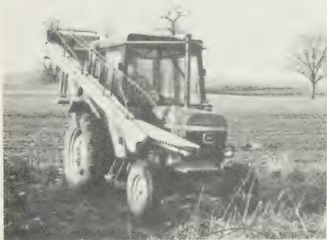
Fig. 16.10 Hop bine loader showing mounting on conventional medium-powered tractor; gathering jaws and bine-gripping chains at front of machine; guard rails to guide 'strings' clear of tractor; and horizontal section of track running to centre-line where the string is tightly gripped and pulled from the overhead wires. (CWF Trumpet)
