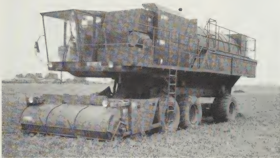
Fig. 16.11 Six-wheel drive low ground pressure pod-picker SP pea harvester at work. (FMC 979).
