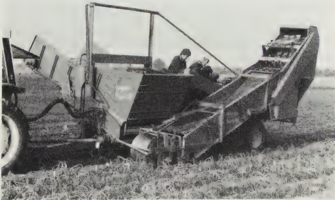
Fig. 15.3 A one-row trailed potato harvester with offset lifting; through-flow haulm separation assisted by spring-loaded rubber fingers; picking table with separate stone and clod conveyor; bunker hopper with hydraulic vertical lift, and unloading-floor conveyor drive. Low draught, good manoeuvrability and minimal tuber damage are reported by users. (Standen/Wuhlmaus ( Sabre TF ))
