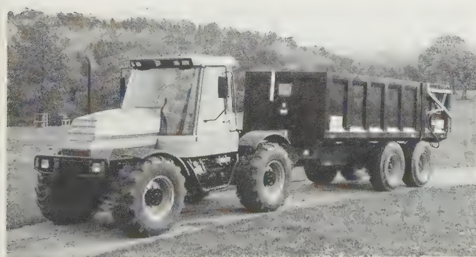
Fig. 21.7 The JCB High Mobility Vehicle with full suspension and air brakes can haul up to 14 tonne loads at 40 mph in a suitable tandem axle trailer engineered to highway duties specification matching that of the tractor. (JCB HMV)
