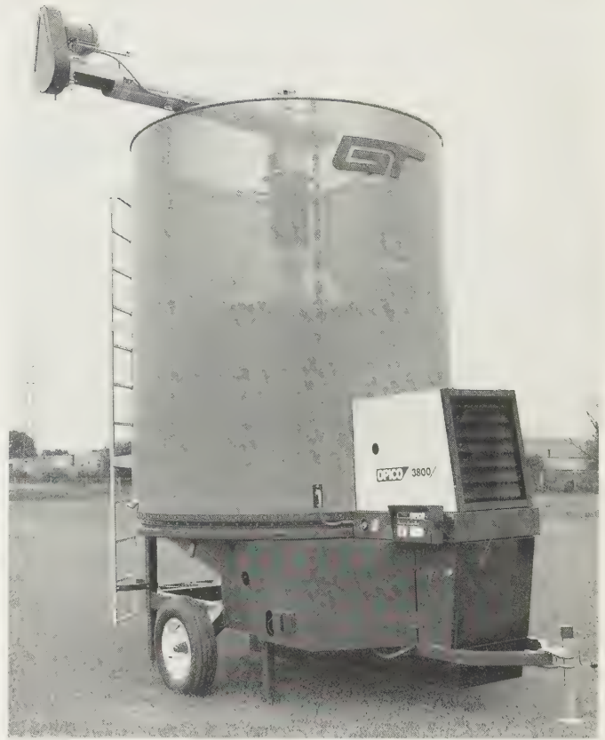
Fig. 18.12 Fully automatic recirculating batch grain drier with DCM control system. Throughput is up to 90 tonnes at 5% moisture reduction per 24 hours. ( Opico Model 3800A )
