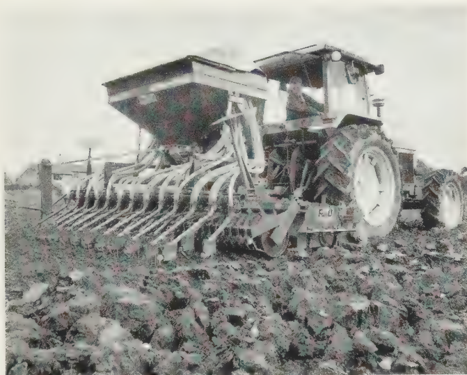
Fig. 3.4 Front-weighted four-wheel-drive tractor with rear-mounted RAU Rototiller and packer-roller producing a seedbed suitable for once-over drilling from rough ploughing using S.A. COMPACTOR Accord pneumatic drill. (Ferrag)
