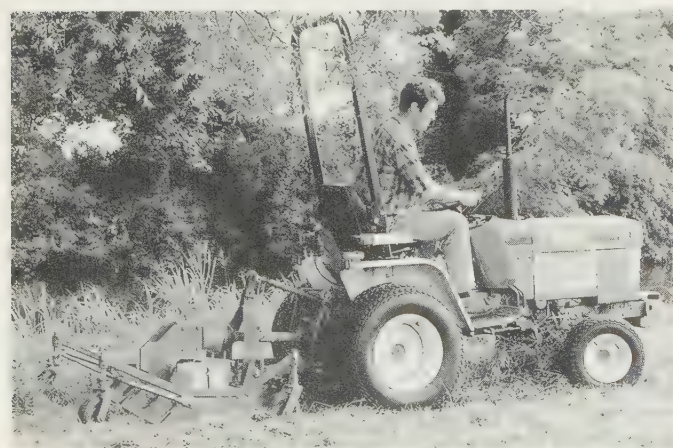
Fig. 16.4 The 1120 11 kW model (14.5 DIN hp) is smallest in the Ford Series 20 Compact range. It is shown here with a sturdy rotary mower designed for use where the going is rough and access difficult. (Ford New Holland)
