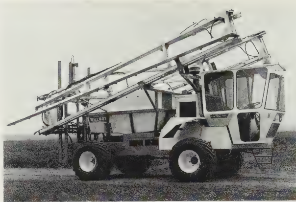
Fig. 2.40 High clearance, lightweight self-propelled sprayer/distributor with 24 m alloy booms designed for easy demounting to fit alternative applications systems. ( Willmot Lightspray )
