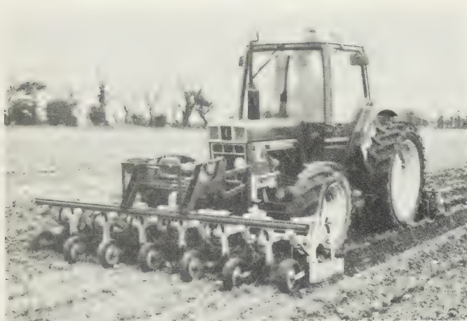
Fig. 6.24 A six-row cultivator/hoe for front or rear mounting, using front-mounted hoes in sugar beet. The heavy lever-action units fitted with side-shields can be self-steered for rear hoeing if suitable marker tines are fitted and used when drilling, and two centre-ribbed wheels used to follow in the grooves created. ( Standen 'Multivator' )
