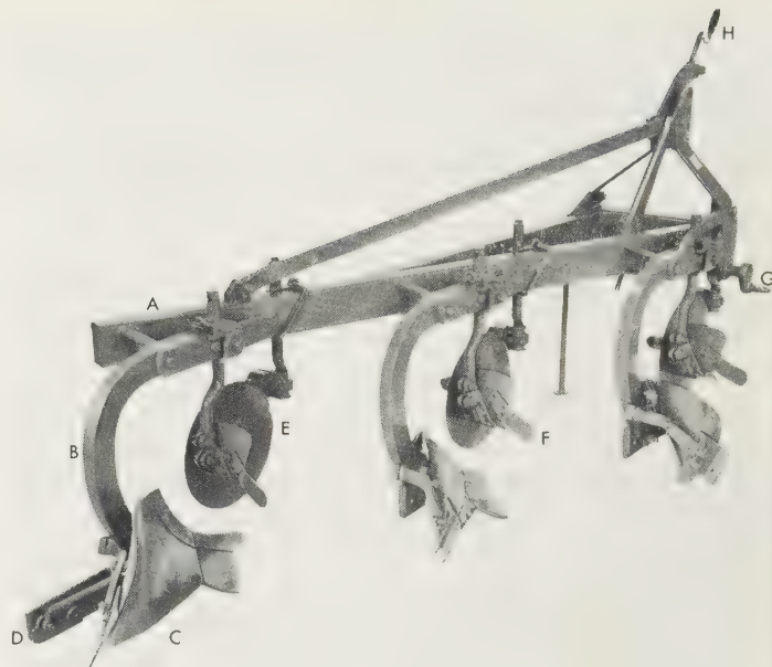
Fig. 4.4 Plough components (Ransomes) A Main frame, B Leg, C Semi-digger body, D Landside and slade, E Disc coulters with tilt adjustment, F Skimmer, G Cross-shaft and hitch pins, H Width control by rotation of cross-shaft.
