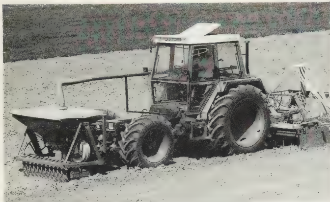
Fig. 2.39 Fendt medium powered four-wheel-drive tractor typical of 1990's trends. The front load platform is capable of carrying a complete 190° slew 8 m reach flail hedge cutter, but is shown here with Accord DF 3 metre Turbo-drill T 300A which has its coulter-bar attached close behind a vertical-axis 3 m power harrow. The seed is carried in the front-mounted hopper, with spiked metering drive wheel and hydraulic drive centrifugal fan conveying metered seed via mushroom seen at rear to the coulter. A wavy-edge crumbler roller levels the between-wheels strip. ( Fendt F380 KOMPACT GT )
