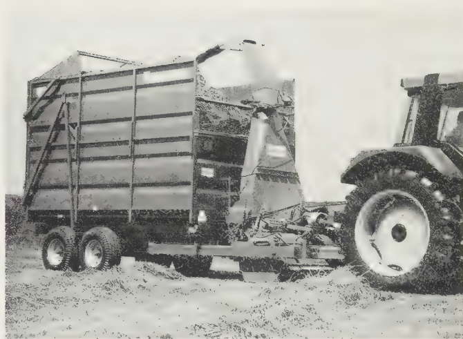
Fig. 12.10 Teagle 'Toucan' at work. Full electric controls. When empty, trailer can easily be separated from harvester and used for normal transport duties. ( Teagle )
