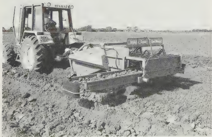
Fig. 7.25 Mounted stone and clod windrower working well in cloddy conditions where two-row beds are to be formed. A set of seven split shares and adjustable discs lift the bed soil on to a steeply sloping agitated digger trace above which an adjustable scrubber trace is suspended. The machine is shown with hydraulic reversible cross conveyor delivering separated clods into a pre-formed deep furrow in which the tractor wheels run on the next bout. (KeyAg Squier 'Clod Master')
