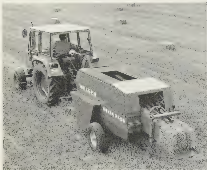
Fig. 13.3 Upper: European small-bale machine using 'in-line' feed system of a general type having affinity with forage wagons and high-density big-balers. Results in terms of neatness of the bales may be seen in the photograph. (WestMac/Welger Delta 2500)
