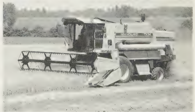
Fig. 14.9 (b) Lateral float headers are now standard on the New Holland models TX 34H, TX 36, TF 42, TF 44 and TF 46. Crop losses at the header are reduced on hillsides and protection provided against bulldozing. (Ford New Holland)
