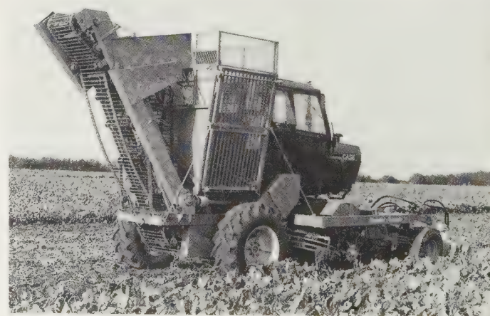
Fig. 15.16 Two-row self-propelled tanker sugar beet harvester based on Case demountable skid unit. Front-mounted hydraulic drive pre-toppers, scalper toppers and wheel lifters are followed by cleaning by rotary 'Cyclone' and Continental web mechanisms. ( Standen 'Tornado' )
