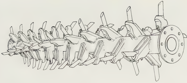
Fig. 6.20 Rotapoint Rotor. The Rotapoint tines are mounted tangentially to the rotor in a heavy-duty forged housing, providing a 'pick' action which will penetrate tough soil surfaces and hard, dry clods. The rotor can work directly into stubble to prepare a seed-bed for oil-seed rape, or after ploughing as a secondary cultivation for cereals. Power requirement is low. Fastening by single nut and bolt is accessible to air-powered spanner.
