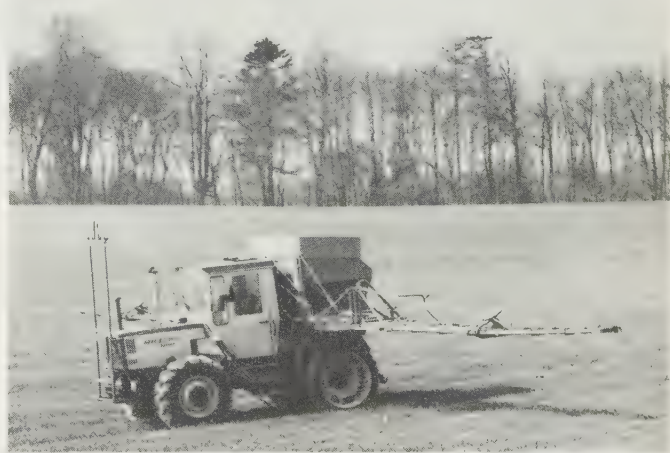
Fig. 8.7 Load platform-mounted 24 metre pneumatic fertiliser spreader with a 'vario-drive' system to enable the driver manually to adjust fertiliser delivery rate to match forward speed. An alternative attachment with microprocessor provides automatic correction for forward speed variations on slopes. The six-section boom is hydraulically folded for transport, with the central sections vertical and the two outer sections on each side running forward above the cab roof to rest on the support at the front of the tractor. ( Amazone )
