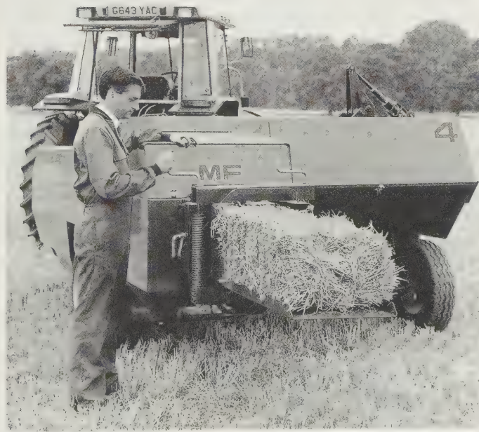
Fig. 13.2 Conventional type of small bale size pick-up baler showing simple adjustment screws for bale tension. Where bales of either hay or straw are intended for dry storage, and the crop is not as dry as desirable at baling, high bale pressure and density may lead to mould development, especially in big bales. (Massey-Ferguson)
