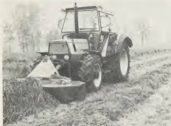
Fig. 11.8 High-powered tractor operating front-mounted and rear-mounted combined drum-and-disc mowers at high speed in a heavy crop. (Watveare/Deutz-Fahr)
