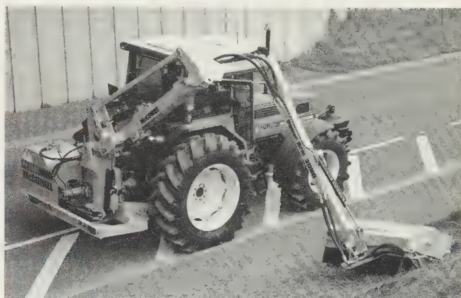
Fig. 22.19 Heavy-duty medium reach flail hedge/verge trimmer rigidly attached to tractor axle by new latch system illustrated in Fig. 22.20. The photograph shows the forward position of the flail head during work. (McConnel PA 2080)
