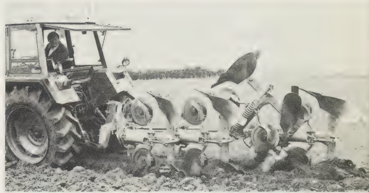
Fig. 5.5(a) Double-link six-ball pivot auto-reset overload release showing high-lift action — position C of left diagram in Fig. 5.5(b).
