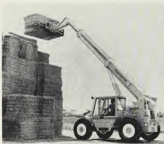
Fig. 13.23 Only a few telescopic boom handling vehicles are capable of good work on the top layer of tall stacks of the biggest rectangular big bales, for example, Hesston 4800 size. The triple extension model seen here has no great difficulty on reasonably level and firm land, but the general demand from farmers who want to use the bales themselves is for one of the intermediate sizes. ( Sanderson Teleporter 2 Model 11-30 )
