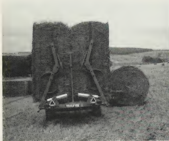
Fig. 13.22 Traileyre System for big rectangular straw bales (Hesston 4800). Equally successful with high-density silage bales produced by medium size big balers. Traileyre handling ability also includes net-wrapped and string tied round and rectangular bales.
