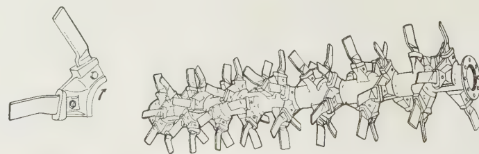
Fig. 6.19 Howard Rotalabour F1 rotor. The F1 rotor is suitable for a wide range of conditions including soils with a high stone content. The knife-tine is retained by a single bolt in a heavy-duty cast steel socket which in turn is welded to the rotor tube. The bolt is easily accessible with an air-powered spanner. The rotor is interchangeable with the Rotapoint type.
