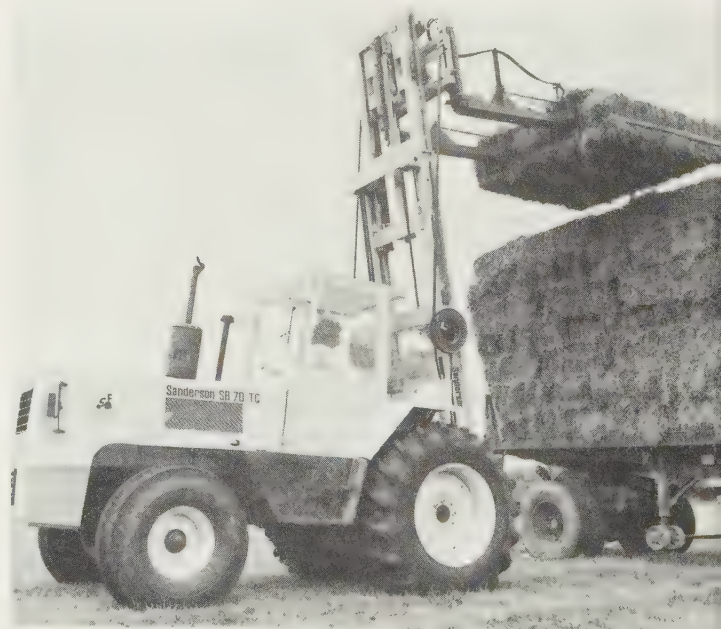
Fig. 13.6 Rough-terrain fork-lift with Triplex mast and 'flat-8' grab attachment loading road transport vehicle. ( Sanderson )
