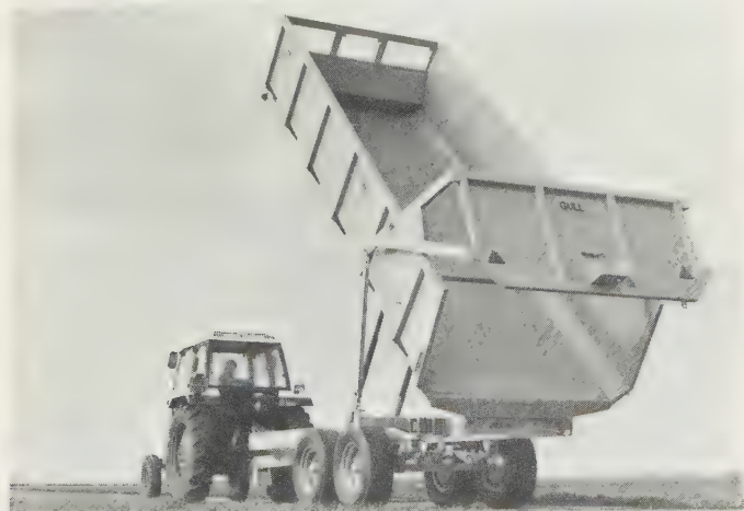
Fig. 21.2 A 10-tonne tipping trailer designed primarily for root crops, having tapered monocoque body with automatic up-and-over tail door, sprung tandem axle and hydraulic cam brakes. (Gull Trailers)
