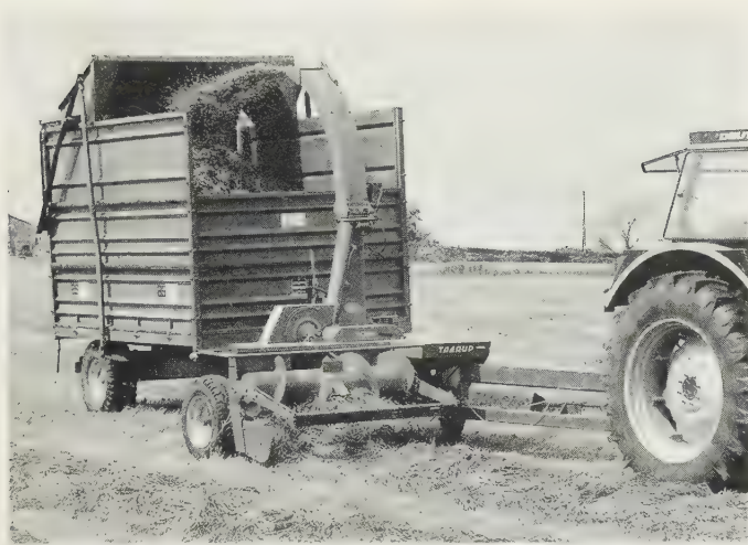
Fig. 12.3 Flywheel type metered-chop forage harvester. Finger-tip in-cab controls provide electro-hydraulic delivery spout movements: instant reverse of feed mechanism to avoid blockage, and trailer tipping. (WestMac Taarup 106B)
