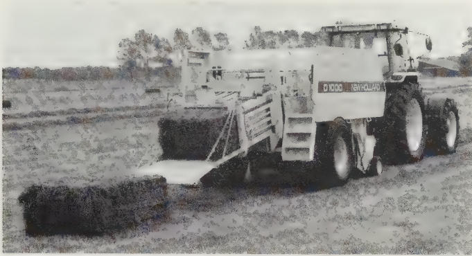
Fig. 13.11 The D1000 Big Baler with advanced Bale Command™ system is able to maintain a high and uniform bale density suitable for silage making with air-tight clamp conservation. The 0.60 by 0.90 m section bales can usefully be made 1.25 to about 1.5 m long for silage and 2.5 m for straw. (Ford New Holland D1000)
