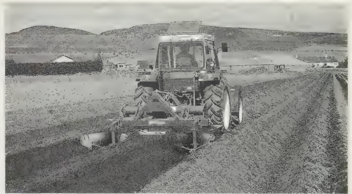
Fig. 7.23(a) The rotary bed tiller comprises a sturdy horizontal-axis rotary tiller with heavy-duty four-speed gear-box and a rotor consisting of spirally arranged hardened steel tines, with adjustable tilth boards for clod shattering. The deep ridging bodies seen are fitted with shear-bolt protection, and for particularly rocky conditions hydro-pneumatic bodies are an option. The equipment can be used in over-wintered or spring-formed beds where cultivation is necessary before stone or clod windrowing. ( Reekie Bed Tiller )
