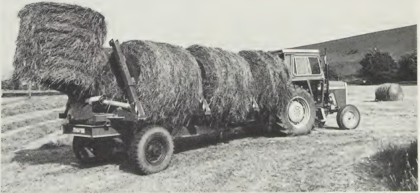
Fig. 13.21 Self-loading bale trailer carrying seven silage bales; six bales are picked up separately at the sides of the vehicle by long spikes carried on hydraulically operated pivoting arms, as
