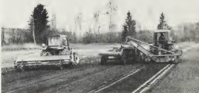
Fig. 22.15 Pto-driven semi-mounted stone rake (left) forming windrows which are picked and loaded by the pto-driven semi-mounted stone picker. ( Kverneland )
