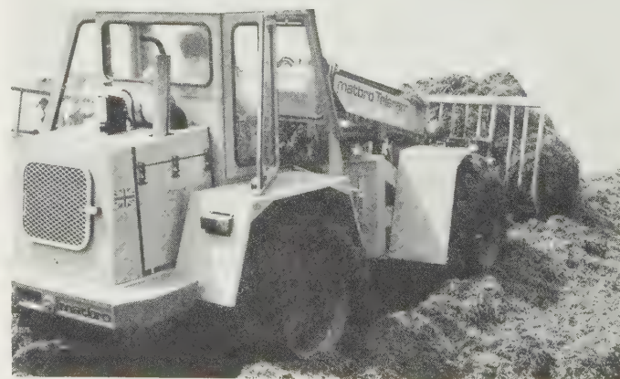
Fig. 21.15 Articulated steer four-wheel-drive telescopic-boom handling vehicle of low overall height with boom lowered, using general-purpose fork to fill clamp silo. ( Matbro 'Telaram' )
