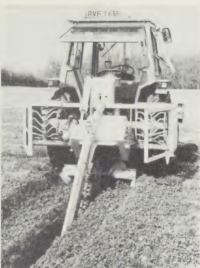
Fig. 22.8 Tractor-mounted pto-driven endless-chain trencher with infinitely variable forward speed provided by a pair of small-diameter cage wheels, driven by the tractor's external hydraulics, and hydraulically pressed into engagement with the tractor's drive wheels during work. (AF Trenchers)
