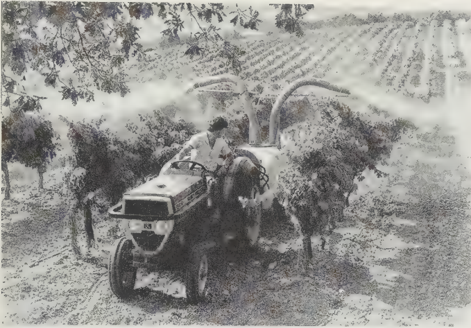
Fig. 16.6 Narrow-track specialist vineyard tractor using air-assisted-delivery sprayer. Work in the narrow rows is assisted by specialist tyre profiles and all-round guards. ( Massey-Ferguson )
