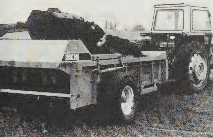
Fig. 8.18 Flail manure spreader with hydraulically controlled rear end-gate attachment to permit handling thick slurry. (S.K.H.)
