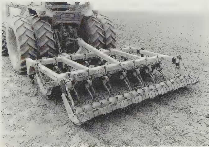
Fig. 6.5 Mounted all-draught cultivator for one-pass seedbed preparation comprising heavy-duty front levelling board adjustable for pitch and designed to cut or crush surface clod; two fully adjustable crumbler rollers of toothed and scraper type. The 350 mm (14 in) diameter front one carries much of the implement weight and is an effective clod crusher; the second of 275 mm diameter levels the soil surface to give reasonable firmness at sowing depth. Two banks of two staggered rows of heavy-duty double-coil spring tines (or rigid straight type) are attached (1) between levelling board and front packer-roller, and (2) between the two packer-rollers. (Simba 'Top-Tilth')
