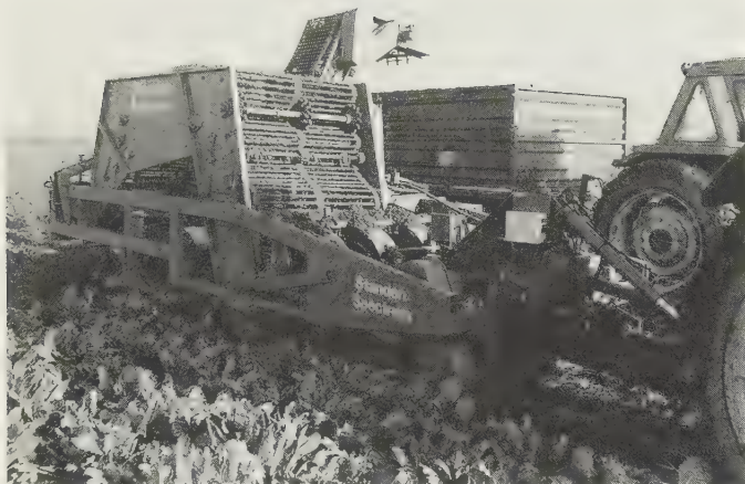
Fig. 15.20 Three-row side-loading trailed sugar beet harvester with open construction allowing wide range of options, as follows:
