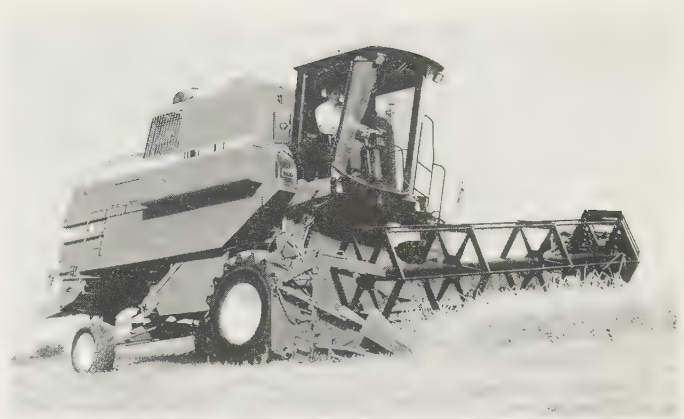
Fig. 14.9 (a) 'Side-hill' combine with provision for automatic levelling on side slopes up to 20% (12° or 1 in 5). Fail-safe outboard disc brakes are fitted. (John Deere)
