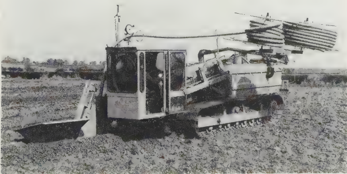
Fig. 22.5 195 kW tracklaying endless chain trencher with independent hydrostatic track drive. Standard features include oscillating tracks, plastic pipe reel assembly, liftable pipe box, and hydraulically supported independent cab. Options include laser depth control, conveyor to remove spoil, and gravel hopper. ( Mastenbroek 26-15 , one of a range of generally higher power and complexity for contract work.)
