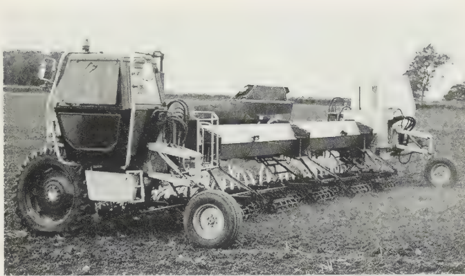
Fig. 3.9 Dowler Gantry prototype trying out pneumatic drill. (Dowler Gantry Systems)
