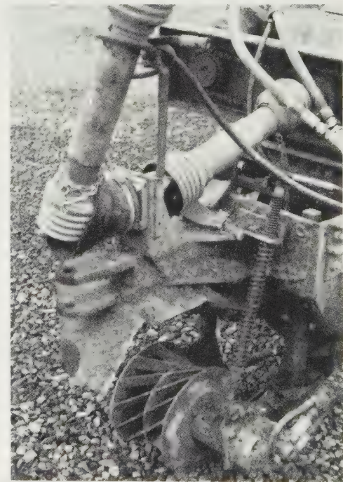
Fig. 15.19(b) Hydraulic-drive 'skew-bar' topper available as option on single-row trailed harvester. (Standen 'Rapide' Mk 3A)
