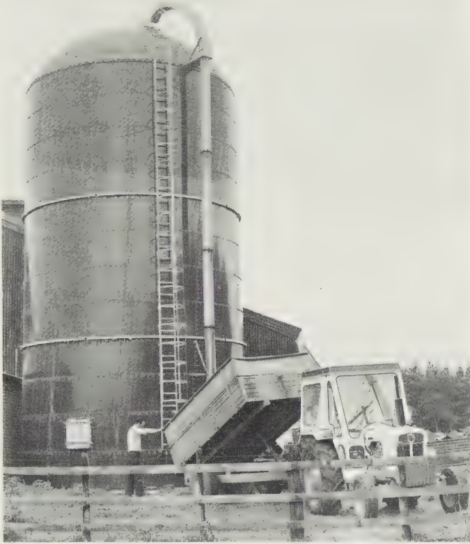
Fig. 18.28 Filling a high-moisture grain store via a tipping trailer and impeller/pneumatic silo filler.
