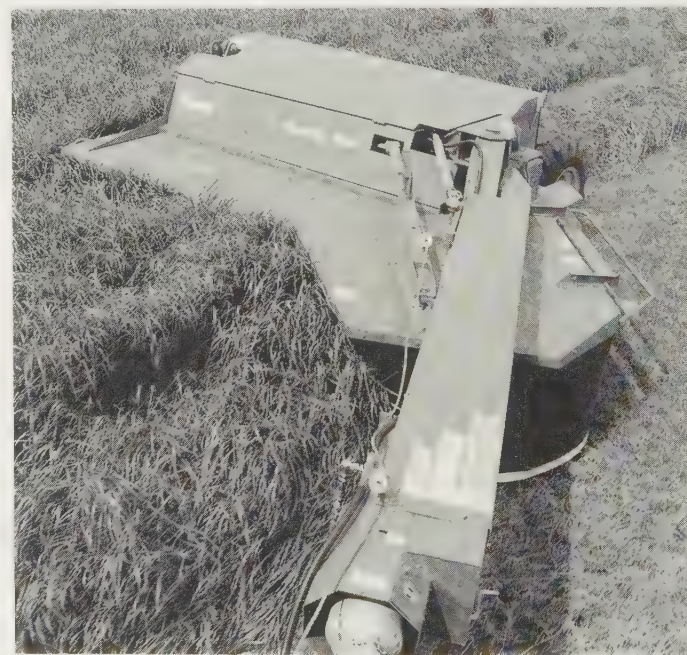
Fig. 11.9(b) View from tractor cab of work done by Clipper 310 mower-conditioner with small third drum working beneath drawbar and driveshaft and one pair of intermeshing nylon brush conditioning rotors handling the three swaths to form a single windrow for wilted silage (Kidd)
