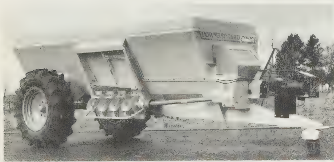
Fig. 8.16 Large capacity farmyard manure/slurry spreader (7250 l, approximately 8 tonnes) with double-taper centre feed auger and wide spreader door designed to secure high discharge rate at low power requirement. The door can be closed down by the single hydraulic ram to reduce application rate; for slurry a narrow door opening can be selected over the full width of the impeller. Deflector plates secure a spread width of approximately 12 m. ( ECON Powerspread 725 )
