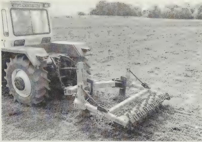
Fig. 5.7 3 m model mounted subsoiler with tine clamps easily adjustable along the main beam to suit individual and varied needs. All tines and teeth have shear bolt protection: tine holes are lined with replaceable hardened bushes. Points and shins are quickly replaceable by removal of two roll pins, and weld-on tips are available for the low-lift points. ( Simba 'Flow-King' )
