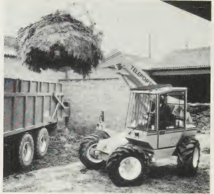
Fig. 21.17 Telescopic boom handling vehicles with four-wheel-drive and steering can make tight turns or move crab-wise on heavy manure handling work in yards originally built for use of hand forks. (Sanderson Teleporter 2)
