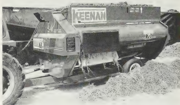
Fig. 12.19 Sturdy Paddle type complete diet mixer feeder with optional electronic weighing for up to 100-cow dairy herd. The massive central paddle rotating at only 10 rpm can produce uniform mix of concentrates, etc., with fairly long silage illustrated. (Keenan Compac 70 Easifeeder)
