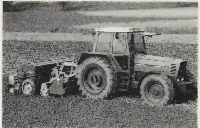
Fig. 3.2 The hinge-linked culti-packer roller and 'Lift-pack' design of the drill lift connections reduces by up to one third the lift force required to raise the drill to a safe position above the packer roller for headland turns and transport. ( Fendt Farmer Turbomatik with Amazone matched power harrow, crumbler and drilling equipment )
