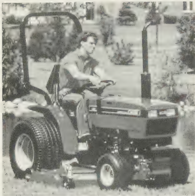
Fig. 16.2 The 17 hp 235, smallest of a range of three models up to 28 hp, is shown with four-wheel-drive and mid-mounted mower suited to well kept lawns or fairways. A wide front-mounted mower of same general type can be used. (Case International)
