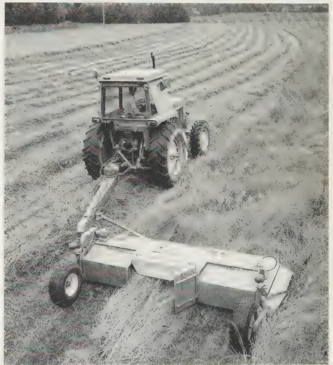
Fig. 11.4 Eight-disc mower of working width 3.18 m with new design narrow wedge-shaped cutter bar carrying triangular three-knife discs arranged to produce a powerful upward air flow. The cut crop is delivered to a high-speed centre-delivery auger rotating at 1400 rpm and producing a powerful air-flow to assist crop conveying. Delivery to the windrow, regulated by adjustable rear doors is by a cylinder of radial fan-type blades built into the centre of the auger. Corrugated bolt-on blade edges work beneath the crop and are designed to produce a stable box-shaped windrow which lies lightly to assist rapid drying and shed light showers. ( VICON ZM 322 Swather )
