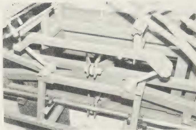
Fig. 9.9 Basic elements of NIAE (now Silsoe Research Institute) pattern boom suspension incorporating a steeply converging pair of V-links, located close to the mast and to the centre of gravity of the boom, which keep the boom substantially parallel to the ground on which the rear tractor wheels stand; and a pair of parallel links, located centrally one above the other and equidistant from the boom centre of gravity, in line with the boom raise/lower cable. These prevent the boom from tilting forwards or backwards. The effect of vertical shocks due to ground irregularity may be minimised by adding shock-absorbers arranged in A form just outside the main V support links. ( Lely 'Autoglide' )
