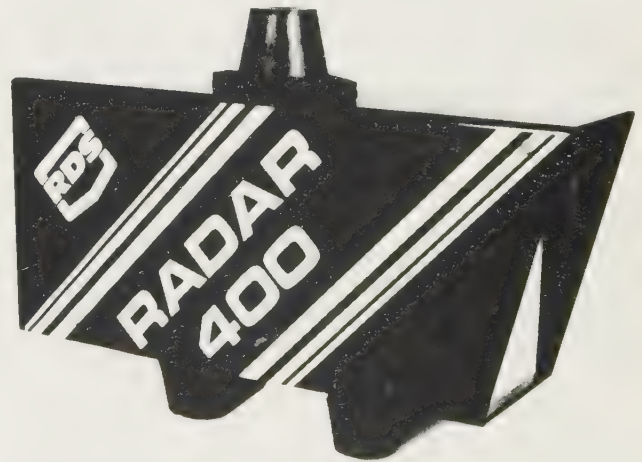
Fig. 2.29(b) Doppler Radar 400 sensor kit (RDS) A low-power signal is directed through the angled deflector to the ground. The reflected signal, mixed with a proportion of the transmitted signal, causes a change in frequency, proportional to the true ground speed, and is in no way affected by wheel slip.
