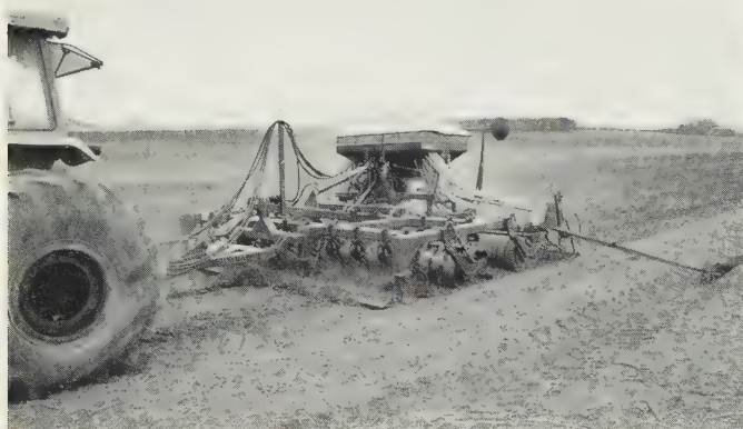
Fig. 3.6 Trailed 4 m seedbed cultivator comprising levelling blade; first spring-tine cultivator row; large diameter toothed crumbler roller; second spring-tine cultivator row; and water ballasted rubber tyred crumbler roller, with rear-mounted Accord DA pneumatic seed drill. The DA is designed for combination mounting on a cultivation implement, often a power harrow. The cultivator model illustrated is operated by a tractor fitted with very wide Terra-tyres, with outside wheel track equal to the width of the cultivator. The combination is moved between fields with the front raised and the implement running on the rubber rear crumbler roller. Wider models can fold wings longitudinally or be end-towed depending on customer preference. ( Simba 'Top-Tilth' with ACCORD DA drill )
