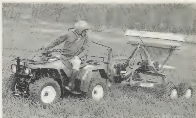
Fig. 8.3 Four-wheel-drive LGP ATVs are increasingly used for early spring distribution of fertilisers on soft wet soils. The Kawasaki and four-wheeled engine driven Logic 40 combination with Vicon distributor is typical of equipment successfully used.
