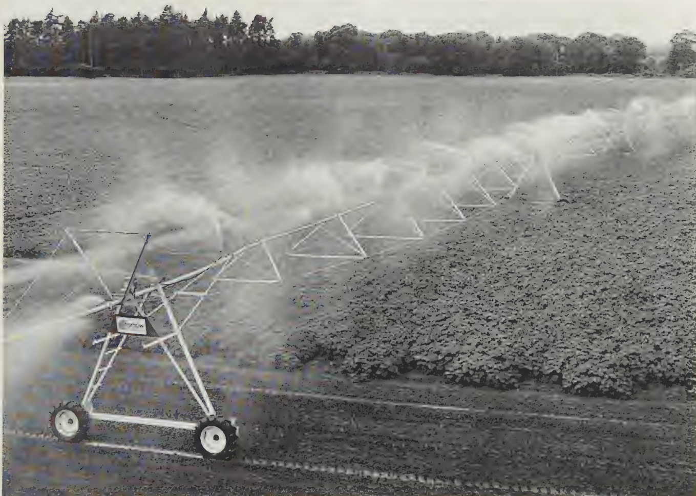
Fig. 10.13 Semi-automatic centre-pivot irrigation system in use in potatoes in Eastern England. After setting up no further manual work is normally needed before harvest. (Wright Rain/Farrow)
