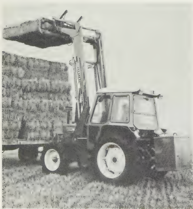
Fig. 13.5 Hydraulically operated bale fork on four-wheel-drive tractor showing high load height capability coupled with adequate reach. ( Farmhand TT Agro )
