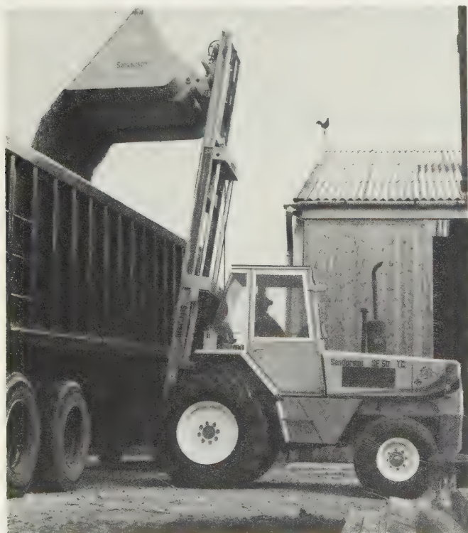
Fig. 18.26 Mast-type rough-terrain fork-lift with grain bucket loading high-sided road transport vehicle. (Sanderson)
