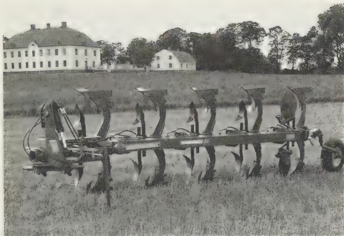
Fig. 5.3 Top of range model from Ransomes RT Hydraulic Auto-reset Reversible Plough range with skimmers, shares and knife coulters designed for use in rocky soils. ( Agrolux )
