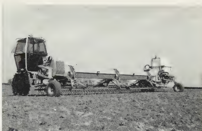
Fig. 3.7 12 m Gantry with three 4 m units of rows of spring-tined cultivator. (Dowler Gantry Systems)
