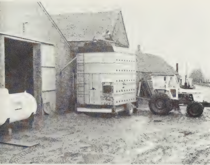
Fig. 18.9 Mobile continuous-flow gas-fired drier operated by tractor pto. Grain is levelled at top by horizontal auger, and flows by gravity over the inverted-V-shaped air ducts. ( Vertec )
