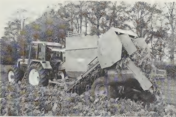
Fig. 15.21 The belt-lift, in-machine-topping system of harvesting sugar beet has been in practical use since Scott-Viner machines were first used in USA in the late 1930s. Modern tractor developments, with ease of providing 75 kW to power the middle-of-range two-row Beaver Super HD illustrated, and particularly to provide the infinitely variable hydraulic drive speeds for the lifting belts and improved cleaning carousels, together with the low-tare and low yield loss of the modern in-machine topping system and 3 m high delivery of crop to the transport trailer, make the current line worth seeing. ( Armer-Salmon Beaver HD )
