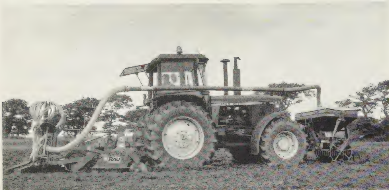
Fig. 1.1 High powered tractor equipped for combined cultivation and drilling operation. The large-capacity front mounted seed hopper is balanced by a heavy Rau rototiller, large diameter packer roller and mounting for the Accord DF pneumatic drill at the rear. Beneath the seed hopper with its spiked wheel driving the seed metering mechanism is a
