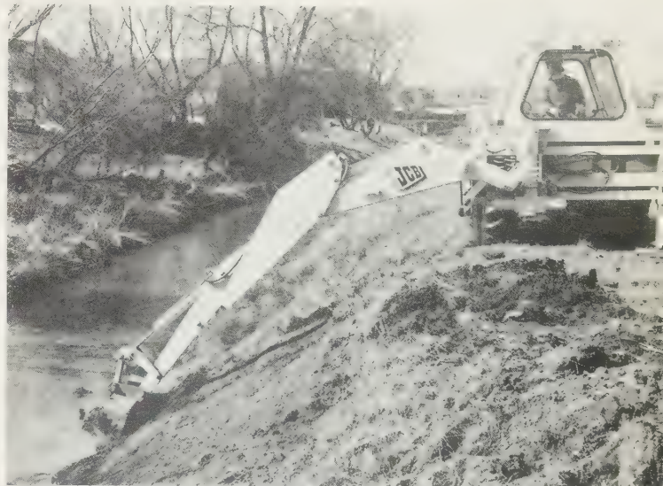
Fig. 22.3 Light-industrial excavator-loader with extending dipper. With swivel-post offset as illustrated the excavator can effectively carry out maintenance on small rivers from one bank only. (JCB)
