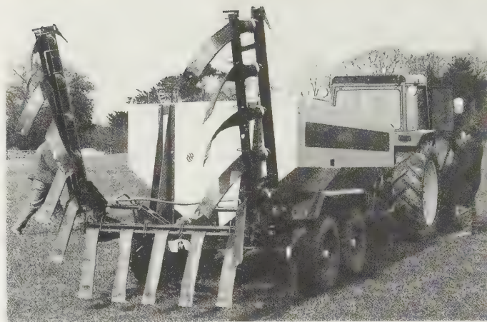
Fig. 8.22 Multi-purpose 7000 l slurry handling tanker shown with 5 m dribble bar applicator hydraulically folded ready for transport (BKW Engineering)
