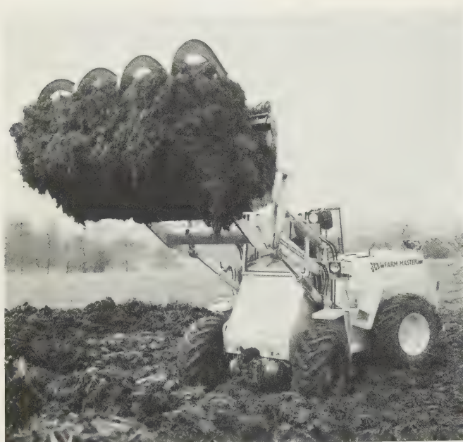
Fig. 8.13 Loading manure from field heap using articulated chassis heavy-duty loader with large grab incorporating push-off. (JCB 'Farm Master')
