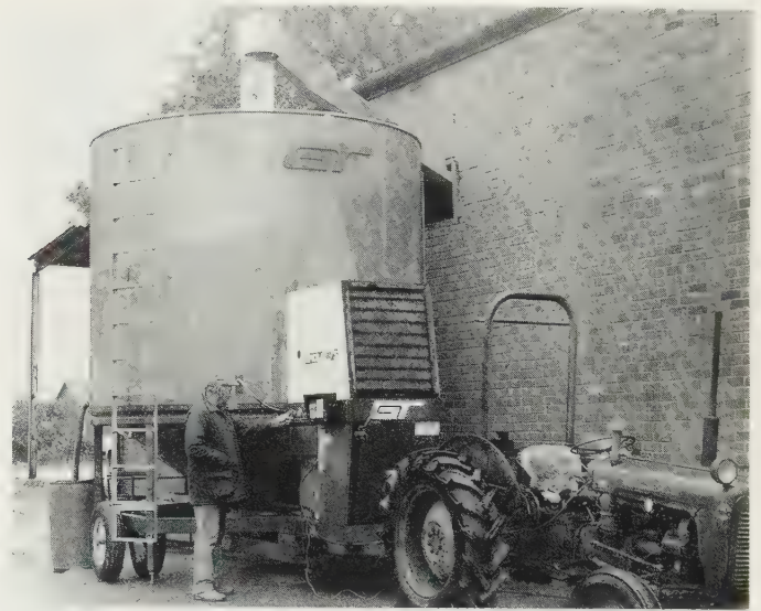
Fig. 18.10 Mobile batch grain drier with pto and V-belt drive to axial flow fan; gas modulating burner; high-speed filling and emptying, and continuous recirculation and agitation of grain during drying. Grain elevated from mobile hopper by horizontal lower and central vertical augers cascades over cone-shaped top of plenum chamber. Drying and cooling air passes from plenum through 46 cm (18 in) cylindrical grain layer to atmosphere. Use out-doors is recommended. Typical drying cycle (including filling and emptying) for 5% m.c. removal is about 2 hours. Automatic controls for end of drying and safety are standard. Batch size of model shown is 500 bushels. ( Opico Model 580S )
