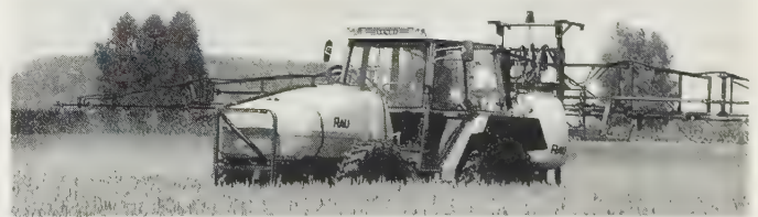
Fig. 2.37 Fendt 380 GT tractor on high-clearance wheels with large spray tank front mounted and rear-mounted sprayer. (RAU)
