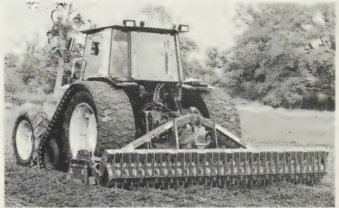
Fig. 6.21 The 4 m power harrow, largest of its range, uses 356 mm (14 in) tines to work the soil to 254 mm (10 in) deep. The harrow is close-coupled to a toothed packer-roller with scraper to prepare a good one-pass seedbed. Power need for high-speed work is met by M-F 3080 fitted with Colmant Cuvelier 'KITCO' rubber wrap-round half-tracks. (Massey-Ferguson)
