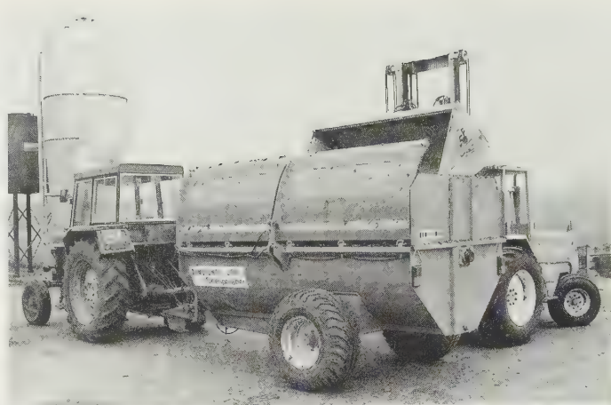
Fig. 8.17 Side-spreader of all-welded rolled steel drum construction with wide hydraulically operated large lid, making it suitable for loading by large bucket or fork. Top-of-range model shown has capacity 6.7 m 3 (8.8 yd 3 ), one-piece forged flail head plates and range of rotor drive sprockets to assist matching to power of tractor used. ( Dowdeswell 2070 )
