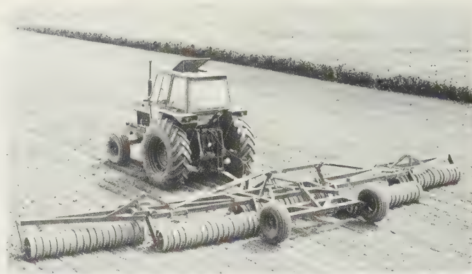
Fig. 6.16 (a) Hydraulically folded 10 m roller with serrated ring sections. Outer sections hinge vertically through 180° to position above inner sections. Outer and inner sections then hinge through 90° and are transported in vertical position. Centre section is raised for transport. (Vaderstad)
