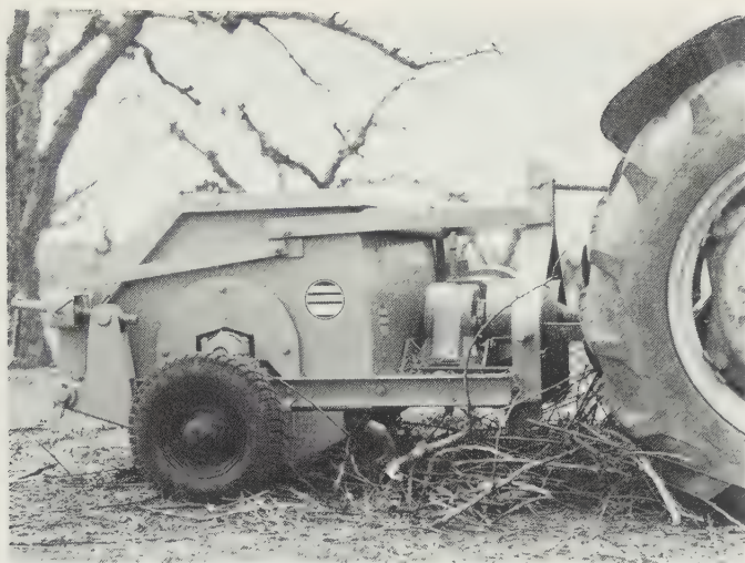
Fig. 16.7 Heavy-duty flail chopper used to pulverise prunings in a grass orchard.
