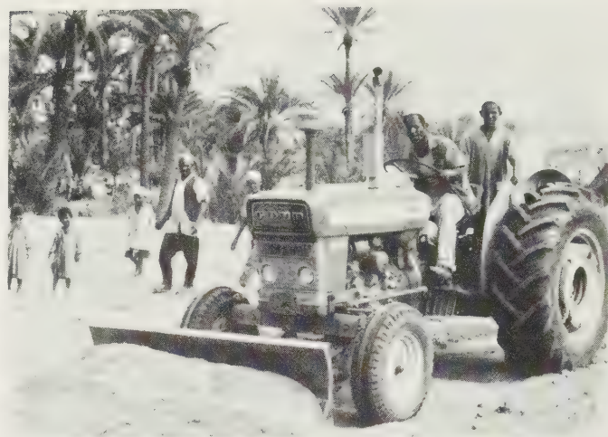
Fig. 22.12 Dozer blade seen on basic tractor (without safety cab). The blade angles 25^\circ either way, tilts 5^\circ , 10^\circ or 15^\circ , and offsets to either side when angled. (Bomford)
