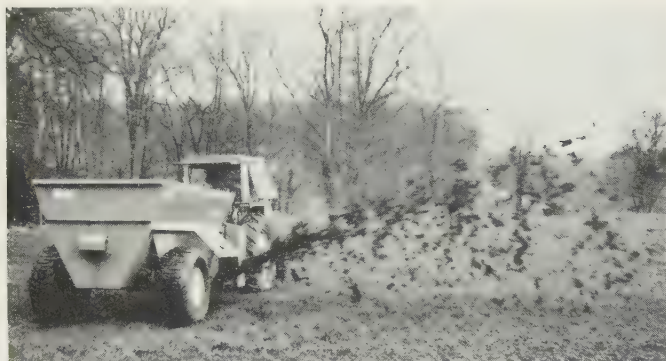
Fig. 8.20 Dual-purpose spreader with flighted conveyor and hydraulically operated sliding gate separating main tank from the high-speed impeller. The machine shown spreading solid manure can also handle slurry. (Kidd 'Tanka-spread')
