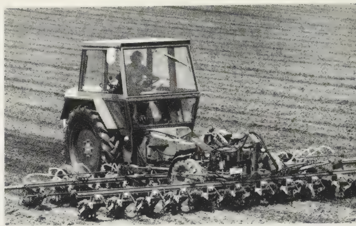
Fig. 6.25 Tool-carrier suitable for 12-row hoeing in crops such as sugar beet, seen here with crumbler roller/drill/sprayer combination. ( Fendt )
