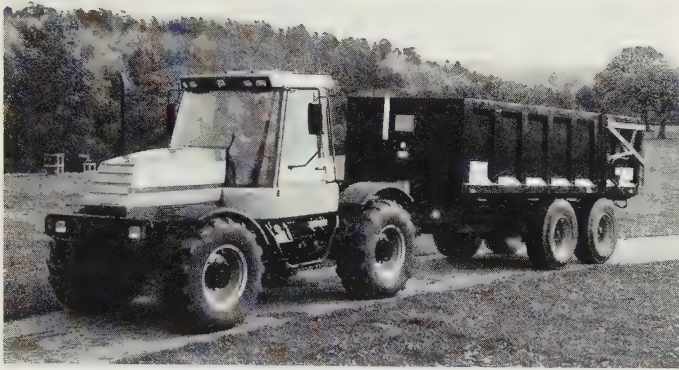
Fig. 2.38 High speed 4-W-D tractor with high speed tandem wheel trailer designed for road speed 40 mph with pay load up to 14 tonnes. (JCB HMV)
