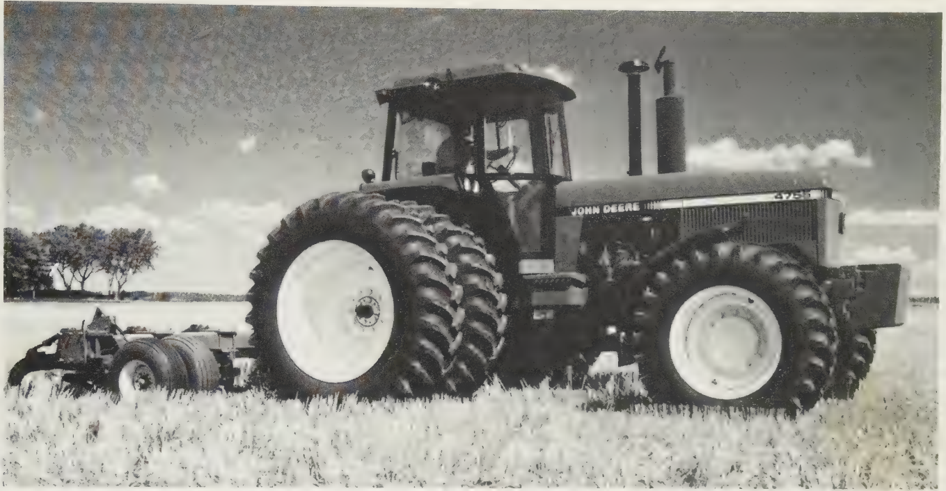
Fig. 1.7 The 190 hp tractor designed primarily for heavy drawbar work is the highest-powered of a range of five which use variants of the same six-cylinder diesel engine. Utilisation of tractors mainly for draught purposes has tended in the second half of the 20th century to be associated mainly with large-scale cereal-growing in areas such as the prairies of North America and the Steppes of Russia in association with fairly shallow disc cultivation and use of discer-seeders. The twin rear wheels with all-wheel-drive and heavy front weights are needed to secure an economic performance using the deep-working cultivator seen here. ( John Deere 4755 )
