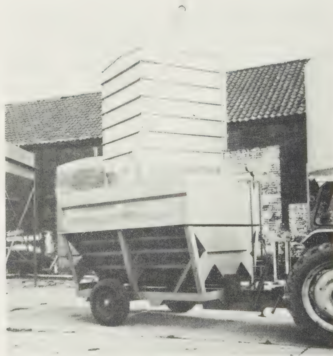
Fig. 19.1 Bulk concentrate conveyor with auger delivery for filling high bulk hoppers. (Rowlands)
