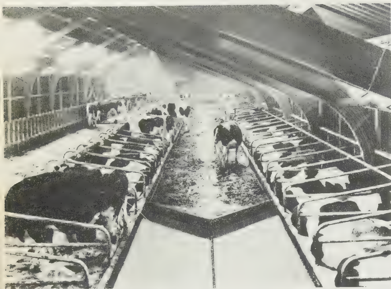
Fig. 8.15 Automatic 'Delta' type winch-operated scraper cleaning a cubicle house. ( Alfa-Laval )
