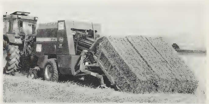
Fig. 13.12 Medium sized square baling system producing big bales 0.8 m square and up to 2.4 m long. The three-bale accumulator is shown in the tipped position and about to release the pack. It is powered by the tractor hydraulics and uses three hydraulic rams, one to position the bales and two to provide the front lift for rapid discharge. The rams are electronically controlled and operation by press button is fully automatic. An indicator screen in the cab displays operating sequence. (Vicon Compact 800 and Browns Big Bale 'Tipper')
