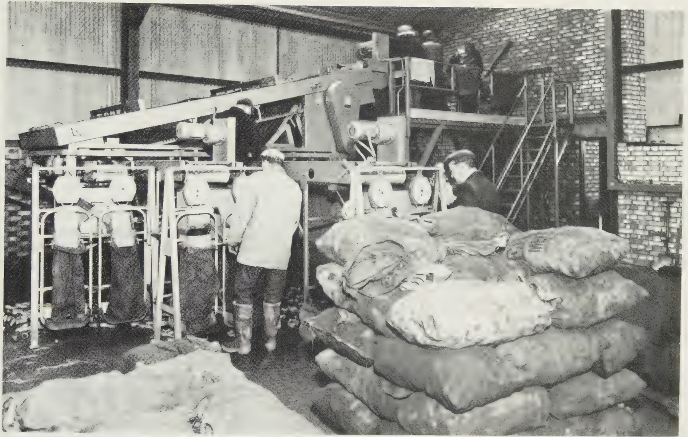
Fig. 16.9 Diverging-roller type of vegetable grader suitable for elongated produce. The installation shown includes belt conveyors and weighing scales for three grades.
