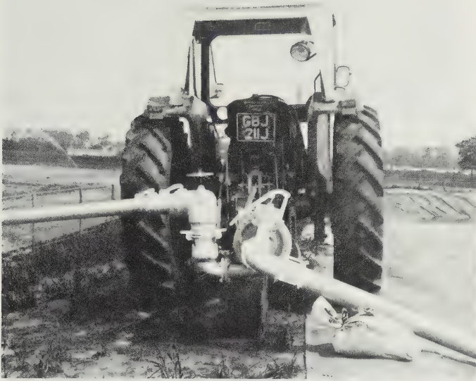
Fig. 10.6 Pto-driven centrifugal pump drawing from butyl-lined reservoir and pumping into portable irrigation main. (Wright Rain)
