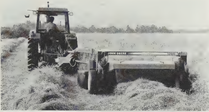
Fig. 11.13 A six-disc 3 m-cut mower-conditioner with heavy free-swinging Y-shaped tines and two-speed drive to rotor by interchangeable V-belt pulleys. (John Deere)
