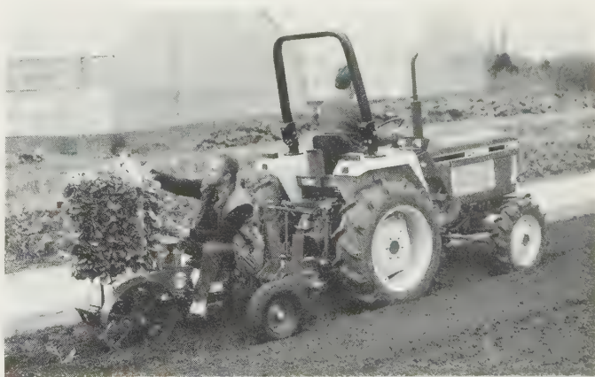
Fig. 16.1 Low-powered 'compact' tractors can be useful for many purposes in commercial horticulture. The axle design (see Fig. 2.45) can provide both four-wheel-drive and good clearance. The three-cylinder model shown operating a transplanter develops up to 27.4 DIN hp (20.5 kW). ( Ford New Holland )
