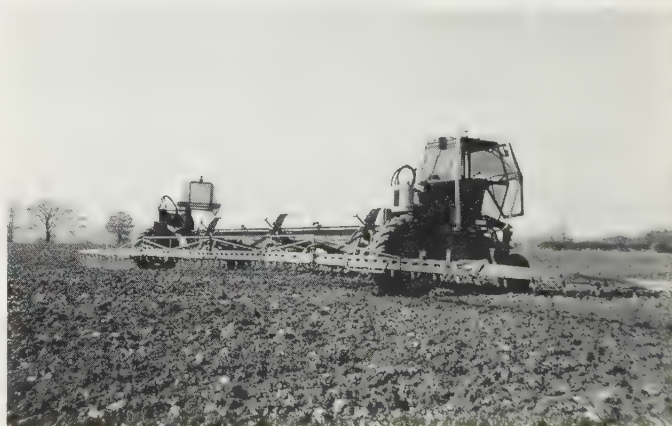
Fig. 3.8 12 m Gantry with sprayer. Two boom extensions make total boom width 24 m (79 ft). (Dowler Gantry Systems)
