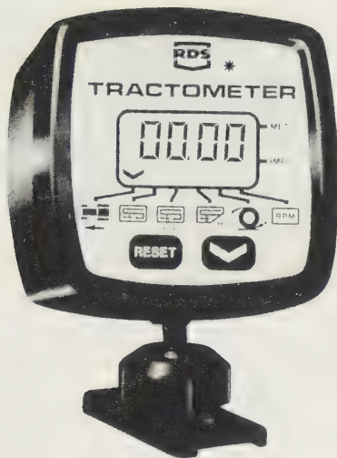
Fig. 2.28 Tractor 2 Performance Monitor (RDS) Display (obtained by touch sensitive pad) gives (L to R) Speed; total area worked; trip area; spot work rate; wheel slip (%) and shaft speed (rpm). Either metric or imperial units can be selected by the operator.
