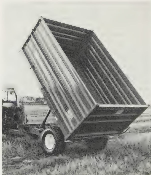
Fig. 21.1 General-purpose 4-tonne tipping trailer with hydraulic brakes and extension sides. (Marston)
