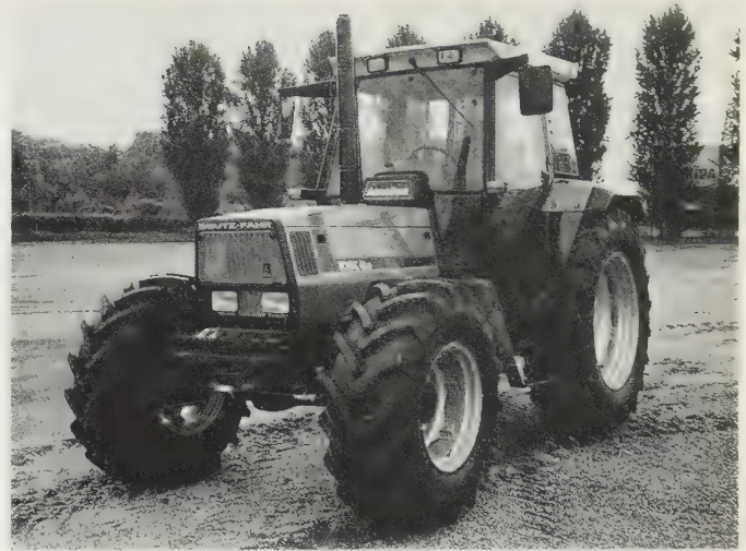
Fig. 1.6 The Deutz-Fahr Agrostar range comprising five models from 88 to 143 DIN hp all with newly designed engines and four-wheel-drive transmission designs resulting in substantially increased engine powers with torque rise up to 26% and an official OECD noise test result of only 72.5 dBA at the driver's ear. The fully synchromesh two-lever transmissions provide up to 48 forward and 12 reverse speeds. (Watveare Deutz-Fahr DX 6.11)
