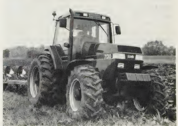
Fig. 2.2 205 hp 7130 tractor from Case-IH 'Magnum' range, operating a Dowdeswell reversible plough typifies the trend to four-wheel-drive, assisted by many efficient modern control features.
