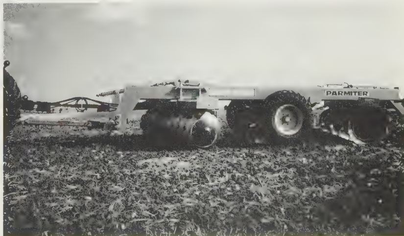
Fig. 6.12(c) Heavy-duty Parmiter UTAH 450 with cut-away discs and hydraulic controls for depth of work and road transport as used for work on stubble breaking on dry land. ( Parmiter )
