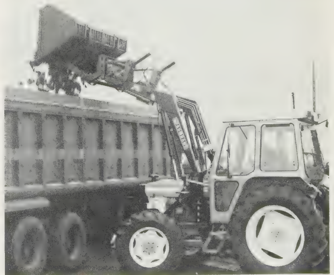
Fig. 21.9 'Toe-tip' bucket, seen on four-wheel-drive tractor loading sugar beet, considerably increases maximum practical loading height compared with bottom hinge type. (Howard G. B. Farmhand)
