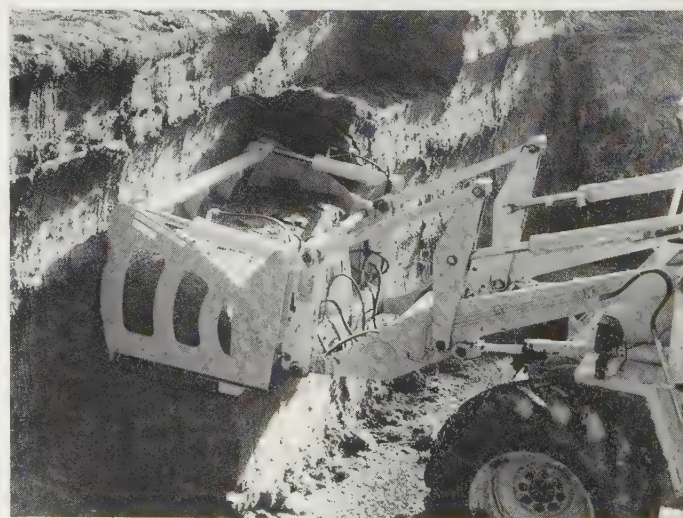
Fig. 12.15 Shear Grab in action clearly illustrates the basic method of use, which leaves the silage face with a smooth and temporarily almost airtight surface, preventing rapid deterioration. (Parmiter SG 300 used on JCB Farm Master)
