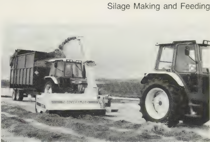
Fig. 12.1 ‘Double chop’ (flail and flywheel chop) forage harvester shown picking up mown swath. Full electric control of spout and deflector from tractor cab is provided. Through drawbar can carry pick-up hitch for loading to trailer drawn in tandem. Harvester can also be used for direct cutting an unmown crop. (Ford New Holland)
