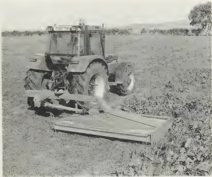
Fig. 11.14 Three-point linkage mounted 2.4 m (8 ft) offset pasture topper incorporating two horizontal steel rotors with a swinging flail angled downwards below the main cutting bar level. A 'thistle basher' blade is standard equipment. A break-back safety linkage is incorporated. Underside of deck is profiled to prevent swathing. ( Kidd Barber 24 )
