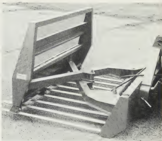
Fig. 12.13 Rear-mounted scissor action push-off buckrake with working width 2 m.
