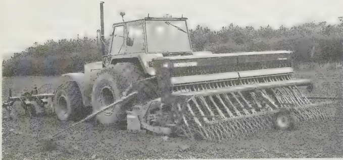
Fig. 7.10 Single-pass 4 m cultivation and drilling by high-powered tractor fitted with LGP tyres operating front-mounted spring-tine cultivator, rear-mounted power harrow and crumbler roller, with Nordsten CLP drill and spring-tine covering. (Howard G.B.)
