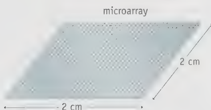
FIGURE 5.3 A microarray. Each dot indicates a position at which a different DNA molecule has been absorbed into the surface of this glass or silicon chip.
