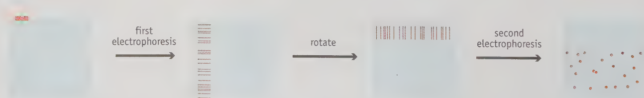
FIGURE 1 Two-dimensional gel electrophoresis.
