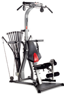
FIGURE 20-17 Commonly found in home gyms, the Bowflex line has become very popular because of its compact, lightweight design. By attachment of multiple rods to the cables, resistance can be increased to provide further challenge. As the rod bends, the tension increases; this is similar to the variable tension created by a band. (Courtesy Nautilus [Bowflex], Inc.)
