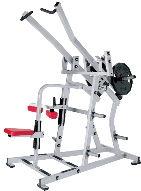
FIGURE 20-24 Leverage machine employing a first-class lever. To use this machine, the client sits on the pad, securing his or her legs under the two pads above. Then, grasping the two handles, the client pulls them downward, raising the weight attached to the opposite end. Much like a playground seesaw, the resistance applied by the client must be enough to overpower the weight attached to the opposite side in order for it to move. (Courtesy Life Fitness, Schiller Park, IL.)
