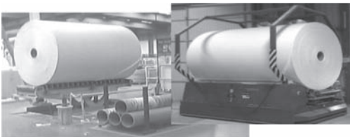
Figure 2. Raw material loading and transport (reels).
