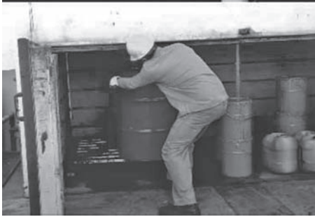
Figure 3. Lack of space to take oil barrel from kiln (support activity).
