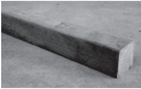
Figure 3. Image of the prototype: Recycled plastic Roof Beam.
