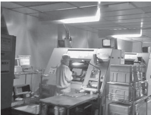
Figure 1. The work environment of light-on test inspection.
