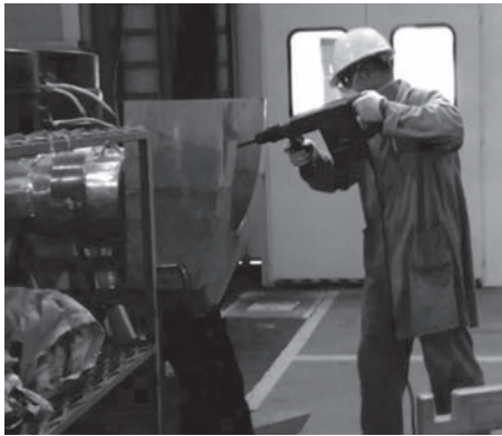
Figure 9. Vibratory tool—support activity cleaning the coke barrel.
