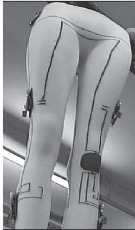
Figure 3. First version of the leggings with the sEMG electrodes and inertial modules, corresponding sensor nodes and data/power tracks made in the textile garment.
